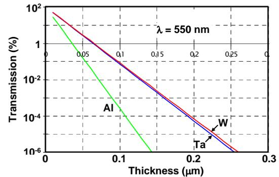
Fig. 4. Light transmission versus lightshield thickness for Al, W, and Ta.
