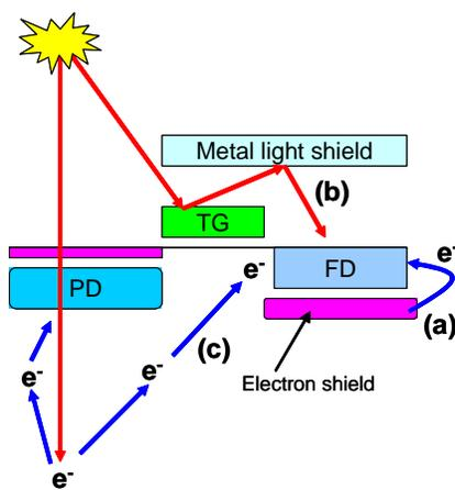
Fig. 2. Mechanisms for floating diffusion leakage in an image sensor with global shutter architecture; (a) junction leakage on floating diffusion (FD); (b) light directly hitting floating diffusion (for example, by scattering off the transfer gate, TG); (c) light hits the photodiode (PD) but absorbs deep in the Si, so it is collected by floating diffusion rather than the photodiode.
