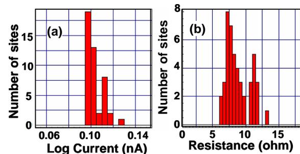
Fig. 6. (a) Gate-to-lightshield leakage and (b) contact resistance for Ta contact to n+ diffusion.
