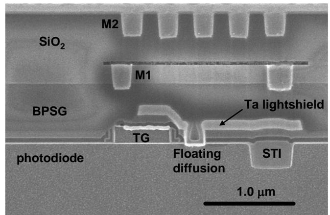
Fig. 5. SEM micrograph of Ta lightshield.
