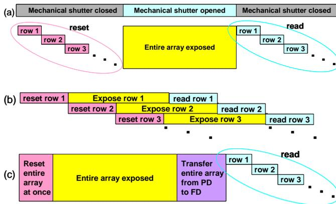
Fig. 1. Schematic of shuttering options for CMOS image sensors; (a) mechanical shutter, (b) rolling shutter, and (c) global shutter [2].
