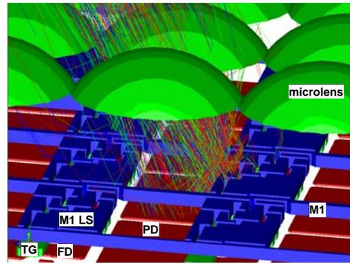
Fig. 3. Simulation of illumination in array with light at 30 degree incidence using M1 as a lightshield.
