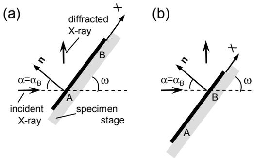
Fig. 2 Diffraction from a chip without warpage. At positions A (a) and B (b), diffraction occurs.
