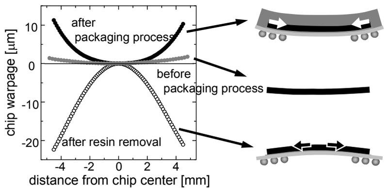
Fig. 5 Chip warpage in a BGA package at each state.
