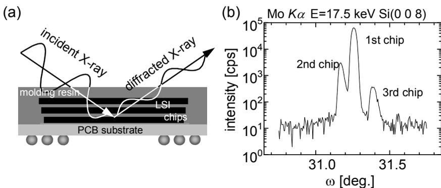
Fig. 6 (a) Schematic image of stacked SiP. (b) Si(0 0 8) rocking curve from the SiP using Mo  $K\alpha$  radiation. Diffracted X-rays from three LSI chips are detected.
