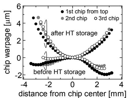
Fig. 7 LSI chip warpage in a stacked SiP before and after high temperature (HT) storage.
