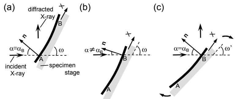
Fig. 3 Diffraction from a warped chip. (a) At position A diffraction occurs. (b) At position B, diffraction does not occur because of warpage. (c) By adjusting  $\omega$  to cancel the warpage, diffraction occurs at position B.
