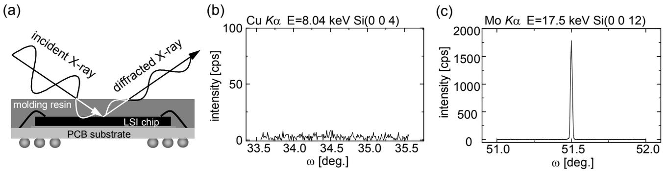
Fig. 1 (a) Schematic image of BGA package. (b) Si(0 0 4) rocking curve by Cu  $K\alpha$  radiation. (c) Si(0 0 12) rocking curve by Mo  $K\alpha$  radiation.
