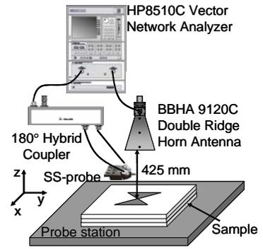
Fig. 3. Experimental set-up.
