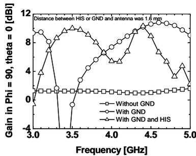
Fig. 7. Gain in the vertical direction versus frequency without GND, with GND and with GND and HIS of 15x15 patches. ( $X = 7.3$  mm,  $g = 1$  mm)
