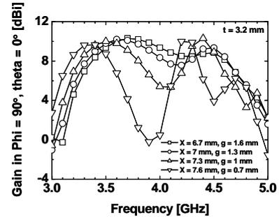
Fig. 9. Gain in the vertical direction versus frequency when patch's widths were 6.7, 7, 7.3 and 7.6 mm for HIS composed with 15x15 patches. (total size = 124.5x124.5 mm<sup>2</sup>)
