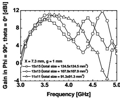
Fig. 10. Gain in the vertical direction versus frequency when the numbers of HIS patches were 15x15, 13x13 and 11x11. ( $X = 7.3$  mm,  $g = 1$  mm)
