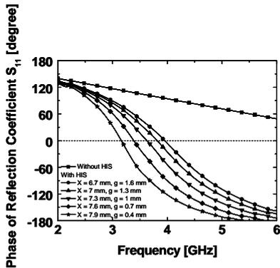
Fig. 4. The phase of S-parameter for reflected wave from HIS.
