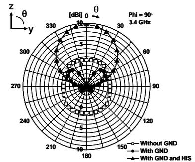
Fig. 6. Effect of HIS and GND on directivity at 3.4 GHz
