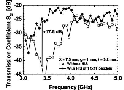
Fig. 12. Measured transmission coefficient  $S_{21}$  versus frequency for the antenna with and without HIS of 11x11 patches at the distance of 425 mm. ( $X = 7.3$  mm,  $g = 1$  mm)
