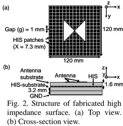
Fig. 2. Structure of fabricated high impedance surface. (a) Top view. (b) Cross-section view.
