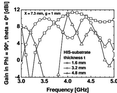
Fig. 8. Gain in the vertical direction versus frequency when HIS-substrate thickness were 1.6, 3.2 and 4.8 mm. ( $X = 7.3$  mm,  $g = 1$  mm)
