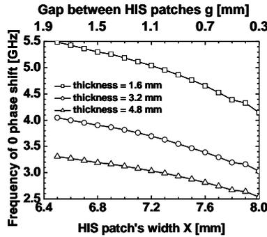
Fig. 5. Frequency for in-phase reflected wave in the function as HIS patch's width and gap between HIS patches.
