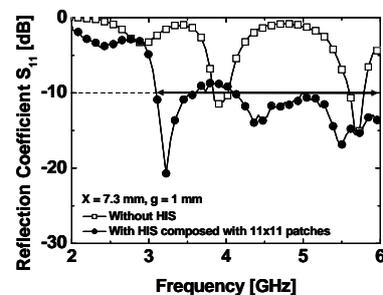
Fig. 11. Measured reflection coefficient  $S_{11}$  versus frequency for the antenna with HIS and without HIS of 11x11 patches. ( $X = 7.3$  mm,  $g = 1$  mm)
