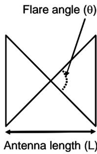
Fig. 1. Bow-tie antenna structure.
