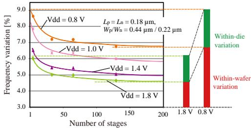
Fig. 3 Stage number and supply-voltage dependence of measured ring-oscillator frequency in the 180-nm CMOS technology. Frequency variations are normalized by the average of the measured oscillation frequency. The effects of within-wafer and within-die variations can be separated with these ring oscillator measurements as indicated on the right side of the graph.
