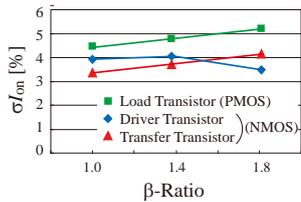
(b) Variations of drain saturation current ( $I_{on}$ ).
