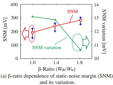
(a)  $\beta$ -ratio dependence of static-noise margin (SNM) and its variation.
