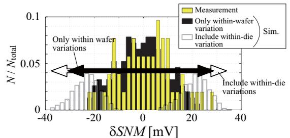
Fig. 6 SNM-variation reproduction with the HiSIM2 parameter set of Table II. Including within-die variations, the measurement data is in good agreement with the HiSIM2 simulation.
