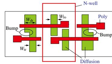
Fig. 4 Layout of the 6Tr-SRAM cell. Bumps of NMOS diffusion are generated by designing for an increased  $\beta$ -ratio.
