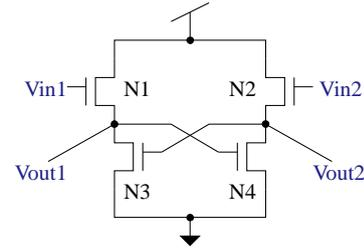
Fig. 1 Schematic diagram of an amplifier stage with feedback coupling (FBC) constructed from NMOS transistors.
