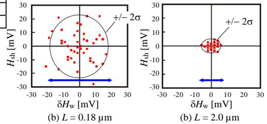
Fig. 2 Hysteresis shift ( $H_{sh}$ ) and width ( $H_w$ ) variation from the measurement of NMOS FBC circuits. Due to only 52 samples,  $2\sigma$  circle is drawn in the graph. The arrow of horizontal direction represents simulated the within-wafer variation from extracted data of single NMOSFET (Table II).
