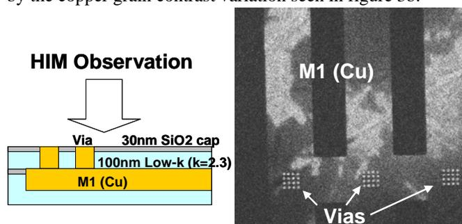
Figure 3a: Side view drawing of copper wiring and its overlying dielectric (left). Figure 3b: CMP power plane seen in HIM SE mode through 130 nm of low-k dielectric material (right). HIM SE imaging conditions were 25 keV and 2 pA and a 20  $\mu\text{m}$  field of view.
