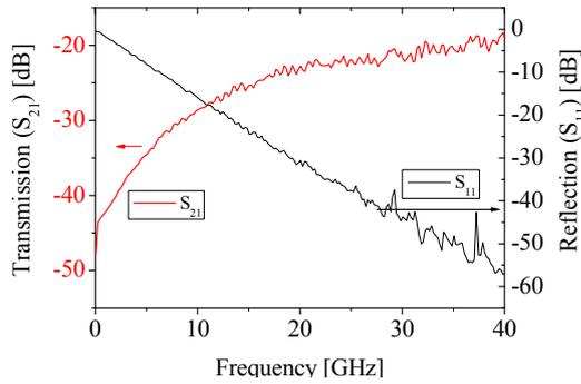
Fig. 3 Measured S-parameter data of a typical CPW with Ge nanowires.
