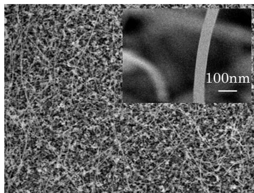
Fig. 1 SEM image of synthesized Ge nanowires.
