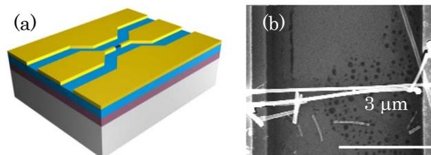
Fig. 2 (a) Schematic of CPWs with Ge nanowires. (b) SEM image of the measured device
