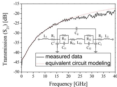
Fig. 4  $S_{21}$  obtained from the measurement data and the equivalent circuit model. The inset shows the equivalent circuit mode.
