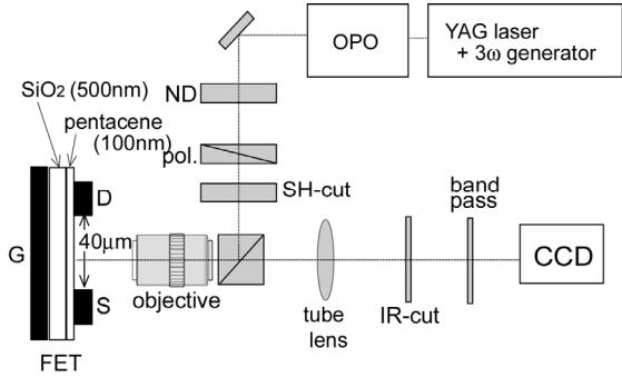
Fig.1 Optical setup for the SHG imaging measurement and the FET structure.
