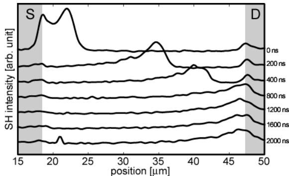
Fig.2 Change in the SH intensity distribution for hole injection.
