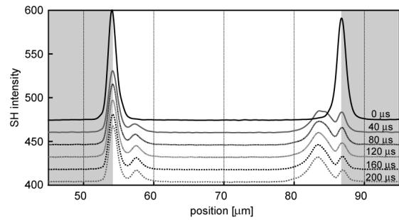
Fig.3 Change in the SH intensity distribution for electron injection.
