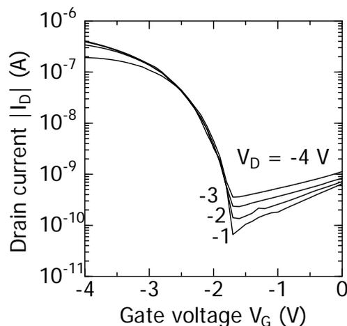
Fig. 3 Gate voltage vs drain current characteristics of  $\text{HfO}_2$  OTFT using deep UV irradiation.
