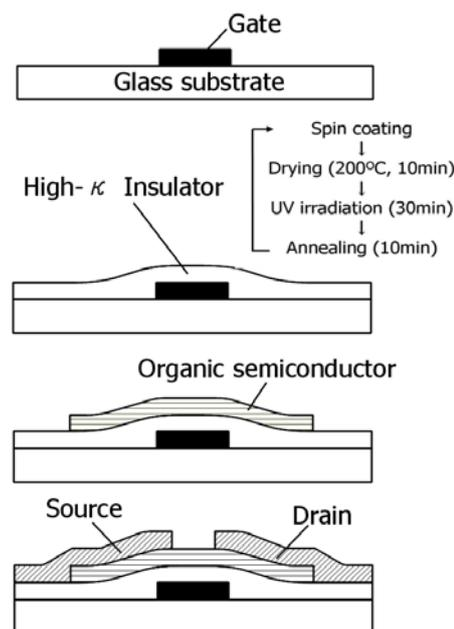
Fig. 1 Fabrication process of OTFT.
