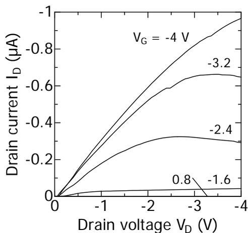
Fig. 2 Drain voltage vs drain current characteristics of  $\text{HfO}_2$  OTFT using deep UV irradiation.
