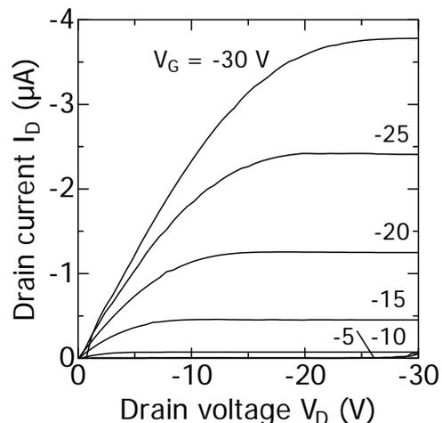
Fig. 4 Drain voltage vs drain current characteristics of  $\text{HfO}_2/\text{Cytop}$  OTFT used deep UV irradiation.
