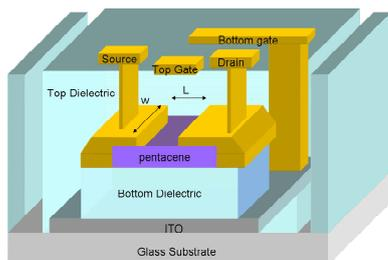
Figure 1 Pentacene OTFTs with double-gate (DG) structure
