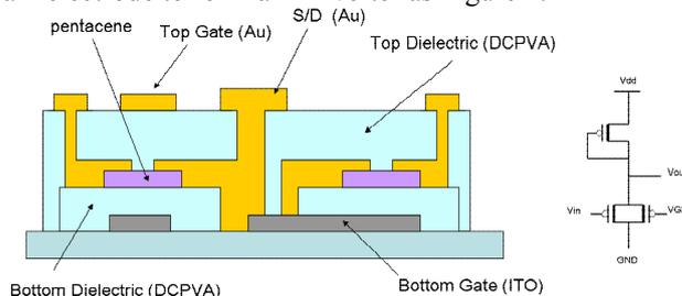
Figure 2 The schematic cross-sectional structures and bias configurations of D-inverter
