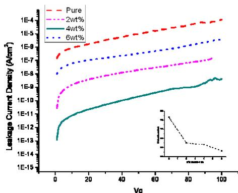
Figure 3 The leakage current of dielectric film with different ammonium dichromate concentrations (an inset that show the dielectric properties of the DCPVA gate dielectric samples with different ammonium dichromate contents)
