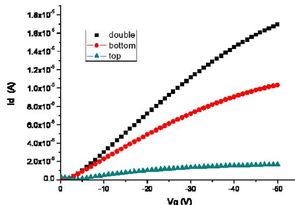
Figure 4 Output characteristic ( $I_{ds}-V_{ds}$ ) for the bottom gate OTFT (circles), the top gate OTFT (triangles) and DG-OTFT (squares) with channel size  $L=50\mu\text{m}$ ,  $W=200\mu\text{m}$ .
