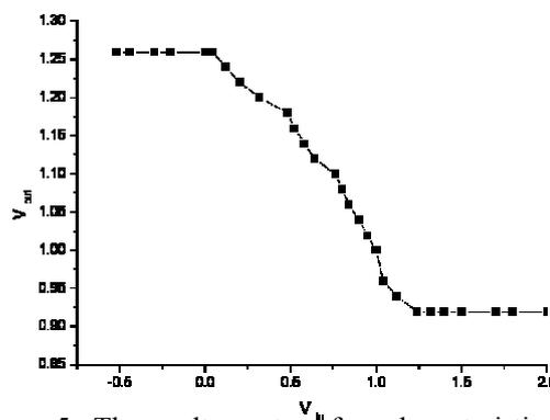
Figure 5 The voltage transfer characteristics of the D-inverter composed of a double-gate driver transistor and a single-gate load transistor as a function of top-gate bias ( $V_{G2}$ ).
