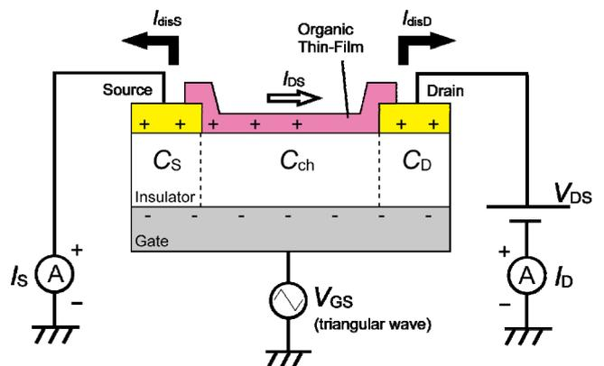
Fig. 1 Schematic diagram of simultaneous measurement method of  $I_{dis}$  and  $I_{DS}$  in bottom-contact OTFTs.  $I_S$  and  $I_D$  are simultaneously measured under the applications of a triangular-wave  $V_{GS}$  and a constant  $V_{DS}$ .
