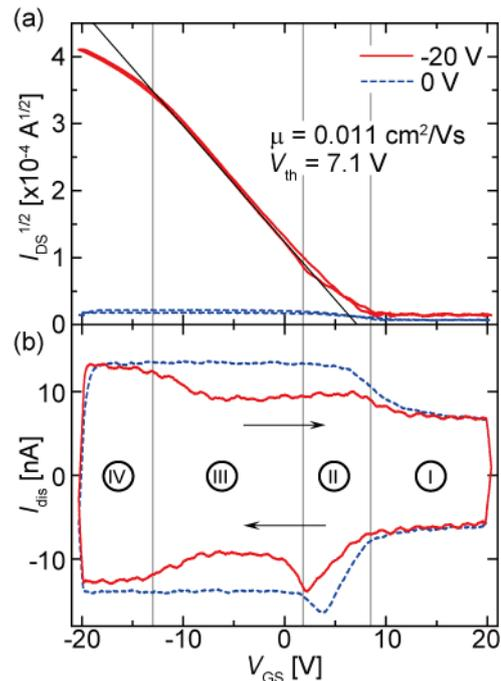
Fig. 2 Experimental results of (a) square-root of channel current ( $I_{\text{DS}}^{1/2}$ ) –  $V_{\text{GS}}$  and (b) displacement current ( $I_{\text{dis}}$ ) –  $V_{\text{GS}}$  characteristics at the  $V_{\text{DS}}$  of  $0$  and  $-20 \text{ V}$  using the simultaneous measurements system.
