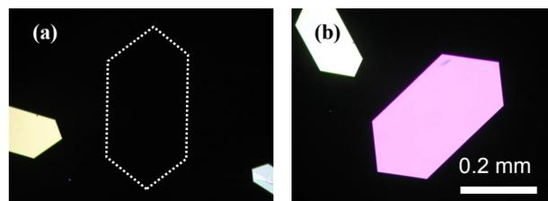
Fig. 2 Polarizing micrographs of an AC'7 crystal. These are taken under (a) the extinction position and (b) the diagonal position of the crossed Nicols. The white dotted line is a guide to eye.
