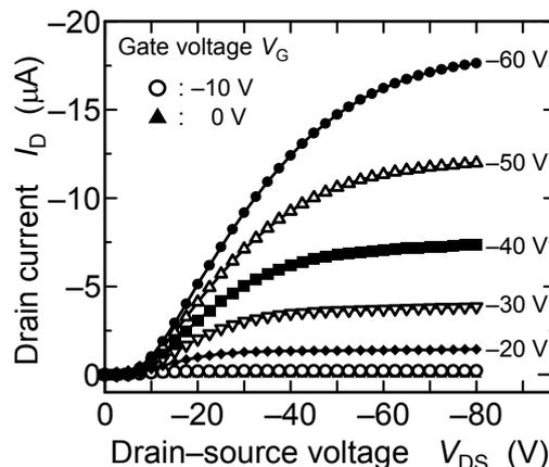
Fig. 4 Output characteristics of the AC'7 crystal OFET fabricated on the SiO<sub>2</sub>/Si substrate.
