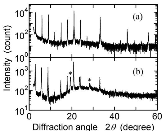
Fig. 3 X-ray diffraction patterns of (a) AC'7 crystals and (b) as-synthesized powder.
