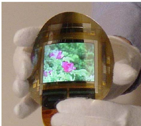
Fig. 4 Photograph of OTFT-driven 2.5-in QQVGA flexible AM-OLED
