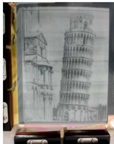
Fig. 6 Photograph of printed OTFT-driven 4.8-VGA flexible AM-EPD.
