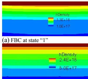
Fig.5 Hole density in the floating body at state "1". Higher hole density is found in the BE-FBC
