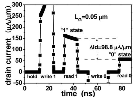
Fig.9 Drain current time dependence during read, write for the BE-FBC with  $L_G=0.05\mu\text{m}$
