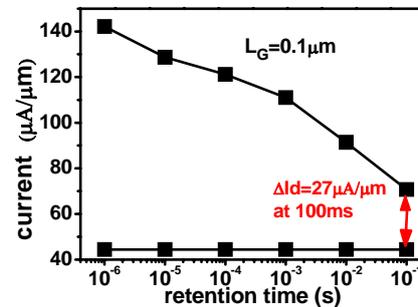
Fig.8 Data retention characteristics of the BE-FBC with  $L_G=0.1\mu\text{m}$  (hold condition:  $V_D=V_S=0\text{V}$ ,  $V_G=-0.5\text{V}$ ,  $V_{BG}=-1\text{V}$ )
