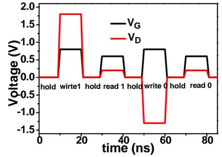
Fig.3 Waveform of the applied biases during reading and writing. The Back gate  $V_{BG}$  and the source  $V_S$  is kept at -1 V and 0 V, respectively.
