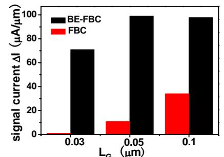
Fig.12 Comparison of the sensing current with different gate length between the FBC and BE-FBC
