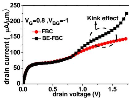
Fig. 4 Output curves of the cells. Kink effect of BE-EBC is clearly seen and more apparent than the conventional FBC
