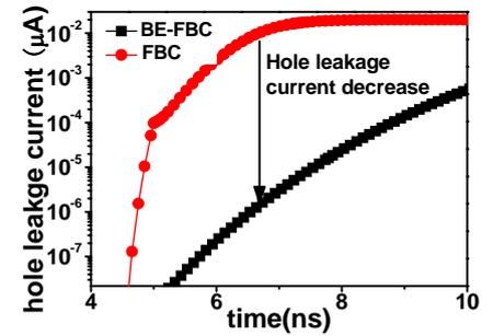
Fig.6 Hole leakage current at the source while applying a writing "1" pulse.
