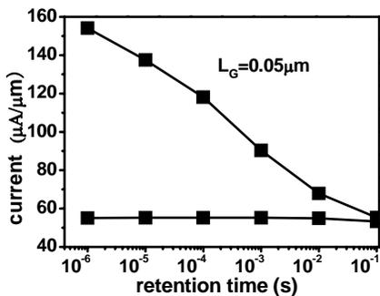
Fig.10 Retention characteristics of the BE-FBC with  $L_G=0.05\mu\text{m}$  (hold condition  $V_D=V_S=0\text{V}$ ,  $V_G=-0.5\text{V}$ ,  $V_{BG}=-1\text{V}$ )
