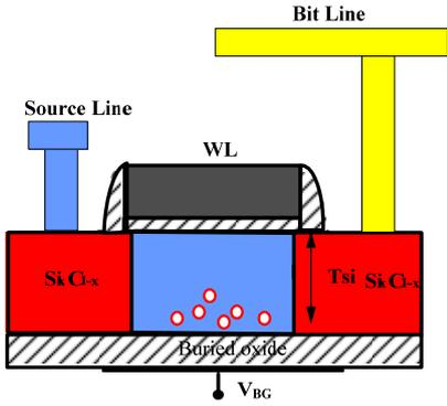
Fig.1 The proposed novel BE-FBC with  $\text{Si}_x\text{C}_{1-x}$  band-gap engineered source/drain.
