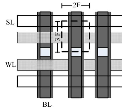
Fig.11 Layout of BE-FBCs,  $6F^2/\text{cell}$  can be obtained.
