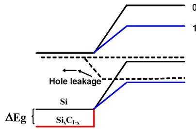
Fig.2 Energy band of the conventional FBC and BE-FBC at state "0" and "1", hole leakage current at state "1"
