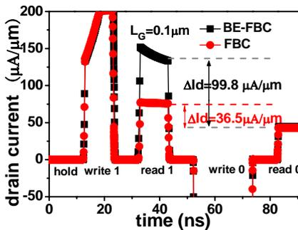
Fig.7 Read and write currents of 0.1  $\mu\text{m}$  cells. The sensing current of the BE-FBC is 3 times larger than the FBC.
