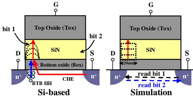
Fig.1 Schematic representation of the cell structure with two-bit storage. CHE and BTB HH injection are used for program and erase, respectively. A reverse read scheme is adopted for two-bit sensing. A rectangular charge with 20nm width is used for charge storage simulation
