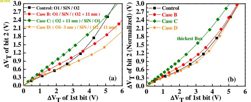
Fig.5 Simulated 2nd bit effect for various cases. (a) w/o, (b) w/ normalized by EOT.
