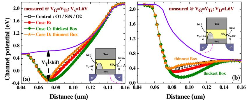
Fig.6 Simulated surface potential for different ONO thickness at (a)  $V_s=1.6V$  and (b)  $V_D=1.6V$
