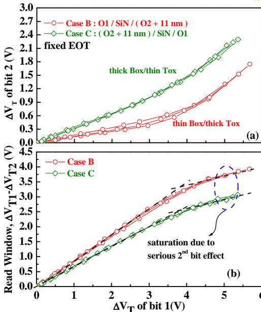
Fig.4 Measured 2nd bit effect for two devices with exchanged Tox and Box (EOT is kept). (b) Read window of Fig. 4(a).
