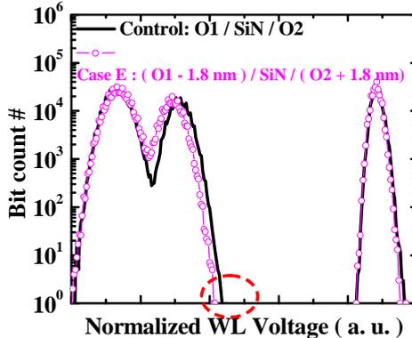
Fig.8 Measured  $V_T$  distribution of a 65nm product. The read window of case E has a 8.5% larger as compared to control sample.
