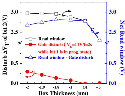
Fig.7 Bottom oxide thickness effect on the net read window (read window-gate disturb). EOT is kept in this study.
