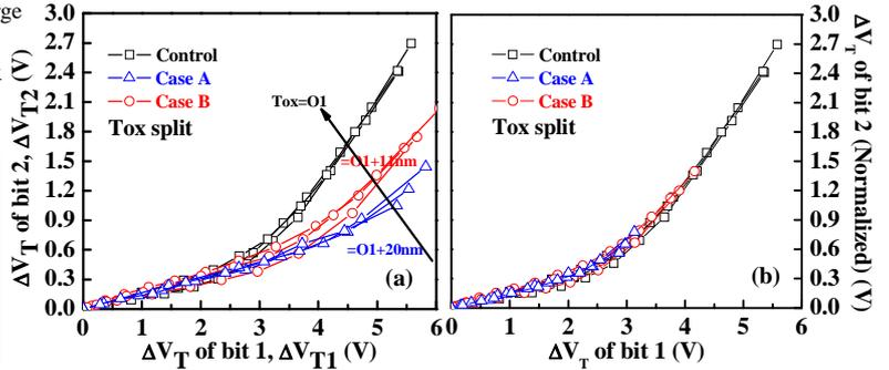
Fig.3 Measured 2nd bit effect for different Tox. (a) w/o, (b) w/ normalized by EOT.
