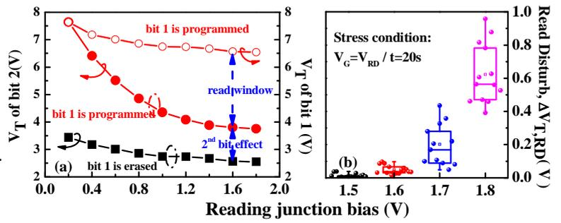
Fig.2 (a) Read junction bias effect on the reverse scheme. (b) Read disturb gets worse with increasing junction bias. Junction bias=1.6V is selected.
