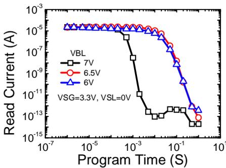
Fig. 4 Program characteristics by channel hot electron injection.
