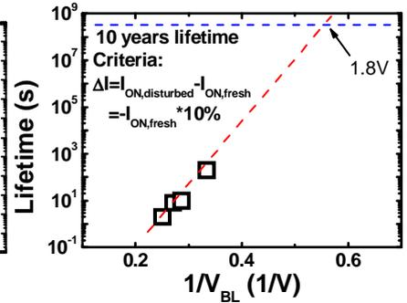
Fig. 6 Read disturb and the lifetime prediction. The cell can sustain continuous  $V_{BL}=1.8V$  DC stress for 10 years
