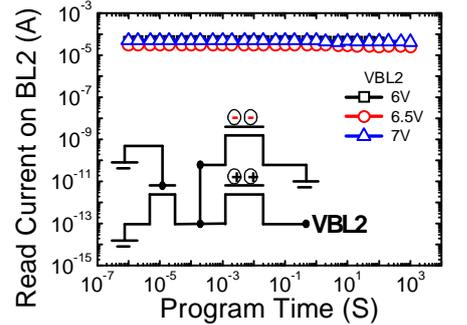
Fig. 3 Self-selective programming on (a) (FG1,FG2)=( $V_{TH,low}$ ,  $V_{TH,low}$ ) (b) (FG1,FG2) = ( $V_{TH,high}$ ,  $V_{TH,low}$ ). After the second step programming, (a) becomes ( $V_{TH,low}$ ,  $V_{TH,high}$ ) and (b) remains ( $V_{TH,high}$ ,  $V_{TH,low}$ ). The two-step program is then finished.
