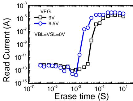
Fig. 5 Erase characteristics at FN operation.
