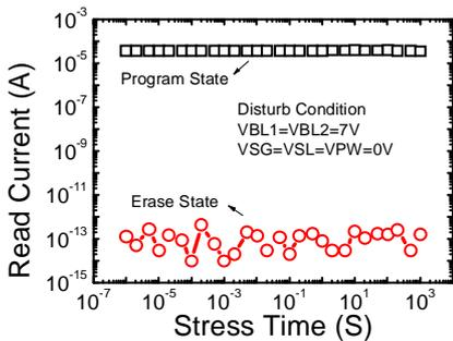
Fig. 7 Drain Disturb on unselected WL. The unselected cell show excellent immunity to high drain voltage over 1000s
