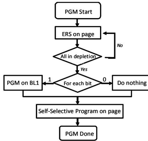
Fig. 2 The new two-step programming scheme.
