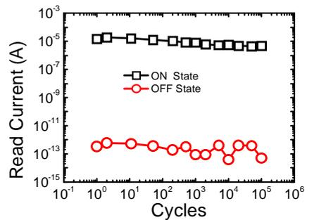
Fig. 9 On-state current is slightly degraded post 100k cycling.
