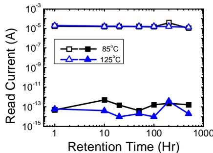
Fig. 8 Data retention characteristics at 85°C and 125°C. No significant charge loss after 1000hr baking at 125°C
