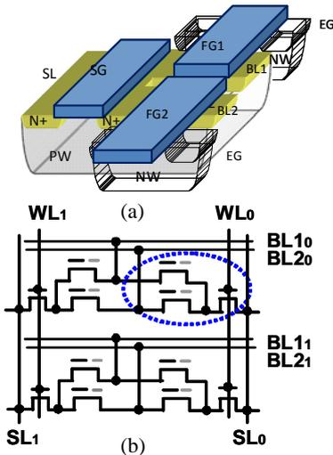
Fig. 1 (a) 3D cell schematics (b) NOR-type array arrangement. The gray line of each transistor denotes the erase gate. Common erase gate connection is not plotted here for simplicity.
