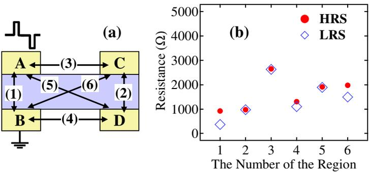
Figure 2 (a) Cross-section of the device with 4 electrode, (b) Resistance of regions (1) – (6) when the resistance of region (1) is switched.
