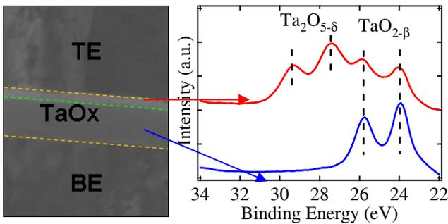
Figure 4 XPS spectra of  $TaO_x$  near the anode and in the bulk
