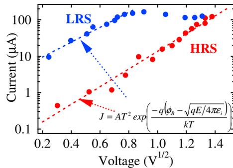
Figure 5 Schottky plot of  $I-V$  curve of a  $TaO_x$  ReRAM memory cell in pulse voltage sweep.
