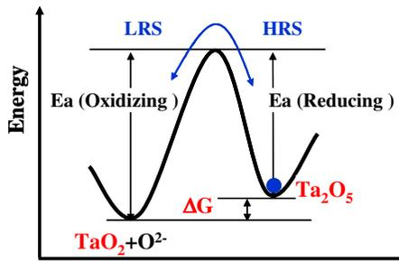
Figure 1 Potential energy curve of  $TaO_x$  redox pair
