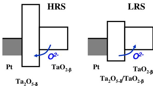
Figure 6 Modulation of the barrier height corresponding to redox reaction
