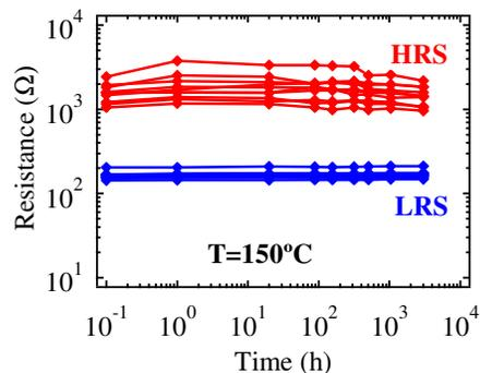
Figure 7 Data retention properties of  $TaO_x$  ReRAM memory cells
