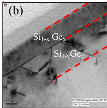
Fig. 3. (a) XTEM of a sample after a 30 nm  $\alpha$ -Ge deposition and annealed at  $950^\circ\text{C}$ , 30s by RTA. Fig. 3 (b) shows a high density defects formation at the interface of  $\text{Si}_{1-x}\text{Ge}_x/\text{Si}$ .
