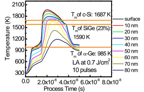
Fig. 5. Simulation of the temperature profile using the heat transfer module of COMSOL Multiphysics. The melt depth induced by LA at  $0.7 \text{ J/cm}^2$  is estimated to be  $\sim 65 \text{ nm}$ .
