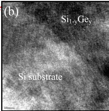
Fig. 2. (a) XTEM of a sample after the deposition of  $\text{Si}_{1-y}\text{Ge}_y$  on Si by UHV-CVD. Fig. 2 (b) shows the high quality and defect free at the interface of  $\text{Si}_{1-y}\text{Ge}_y/\text{Si}$ .
