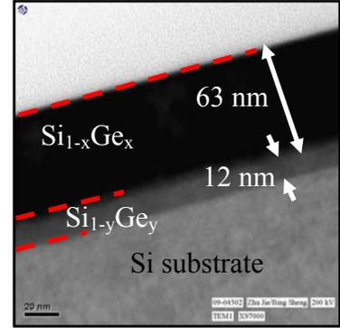
Fig. 4. XTEM of a sample after a deposition of 30 nm  $\alpha$ -Ge and annealed by LA at  $0.7 \text{ J/cm}^2$ , 10 pulses. No observable defect formed at the  $\text{Si}_{1-y}\text{Ge}_y/\text{Si}$  interface. The melt depth induced by LA is  $\sim 63 \text{ nm}$ .
