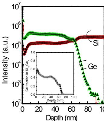
Fig. 6. SIMS profiling shows the Si and Ge atoms depth profile in the sample annealed by LA at  $0.7 \text{ J/cm}^2$  for 10 pulses. The inset shows the Ge concentration extracted by SIMS.
