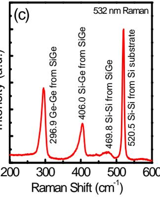
Fig. 7. 532 nm Raman spectrum of (a) as-deposited sample; (b) sample went through RTA at  $950^\circ\text{C}$  30s; and (c) sample went through LA at  $0.7 \text{ J/cm}^2$  for 10 pulses. The peaks from the  $\text{Si}_{1-y}\text{Ge}_y$  layer in the as-deposited sample (a) are too weak to be detected.
