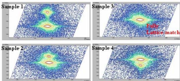
Fig. 1 RSM mapping on the asymmetric (1 0 5) crystal planes for the AlInGaN epilayers prepared in this study.
