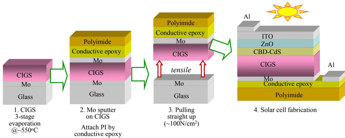
Fig.1 Schematics of lift-off process.
