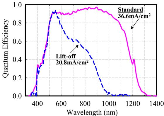
Fig. 4 QE of lift-off CIGS solar cell.
