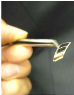
Fig. 2 Photograph of flexible lift-off CIGS solar cell.
