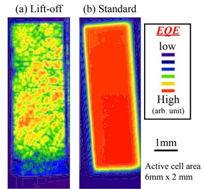
Fig. 5 QE spatial distribution of lift-off CIGS solar cell.
