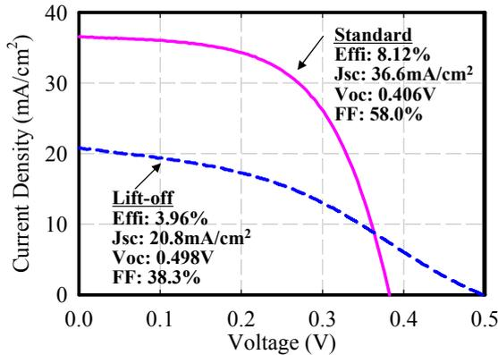
Fig. 3 Current-voltage curves of lift-off CIGS solar cell.
