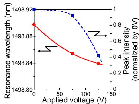
Fig. 9 Applied voltage dependence of resonance wavelength and peak intensity.
