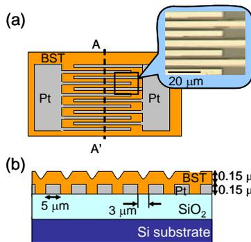
Fig. 5 (a) Schematic plan view and optical micrograph, and (b) A-A' cross section of (a) for lateral-epitaxy sample.
