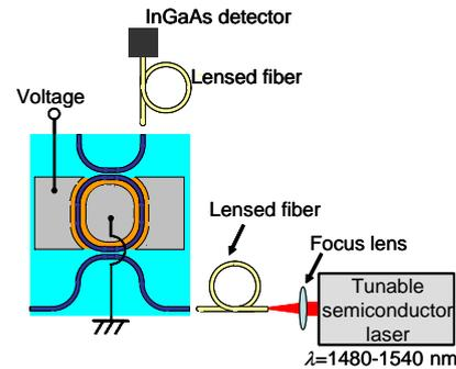
Fig. 3 Measurement setup for characterization of Si ring optical modulator.
