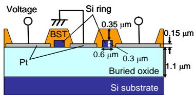
Fig. 2 A-A' cross sectional schematic structure of Si ring optical modulator.
