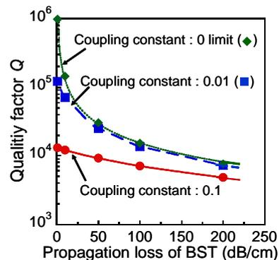
Fig. 12 Calculated quality factor of ring resonator with BST clad vs propagation loss as a parameter of coupling constant.
