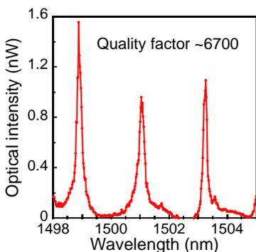
Fig. 7 Resonance characteristics of the fabricated optical modulator with BST clad. The quality factor is about 6700.
