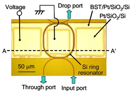
Fig. 1 Typical example of optical micrograph of fabricated Si ring modulator.
