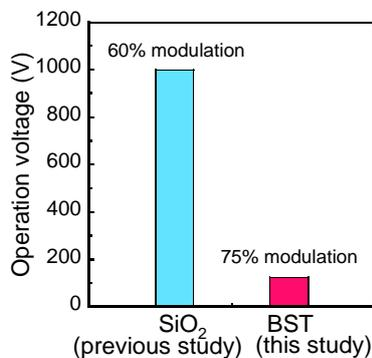
Fig. 11 Operation voltages at 60 % modulation for SiO<sub>2</sub> clad and 75 % modulation for BST clad.
