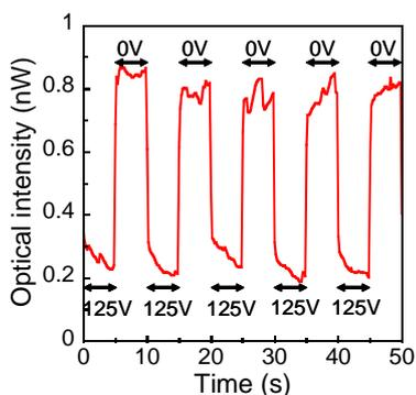
Fig. 10 Optical output intensity at applied voltages of 125 V and 0 V. Modulation is ~75 %.
