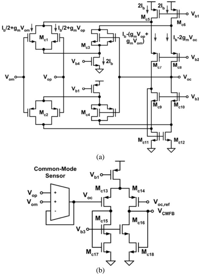
Fig. 4 Proposed CM sensor (a) and entire CMFB circuit (b).
