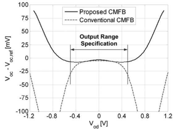
Fig. 5 Relationship between  $V_{od}$  and CM voltage error ( $V_{oc} - V_{oc,ref}$ ) for the conventional and proposed CMFB circuits.
