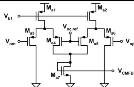
Fig. 3 Conventional current-steering CMFB circuit.
