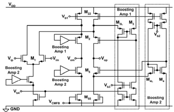
Fig. 1 Gain-boosted folded-cascode OTA.
