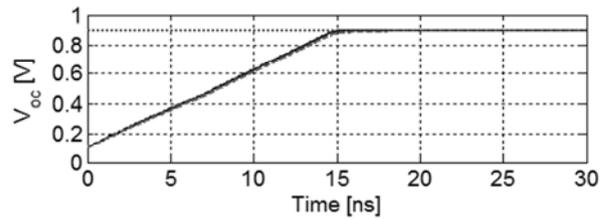
Fig. 6 Settling behavior of the proposed CMFB circuit.
