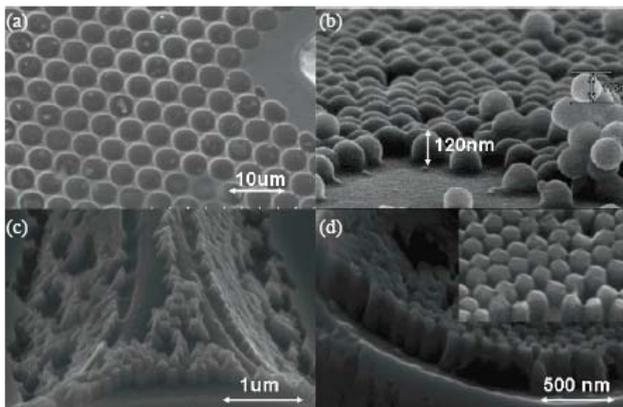
Fig. 3. The SEM figures of (a) The micro-bowls array texture on LED-II surface. (b) The silica nano-particles were spin-coated on surface. (c) and (d) The nano-rods were formed through wafer surface including bowl bottom, bowl sidewall, and plane surface.
