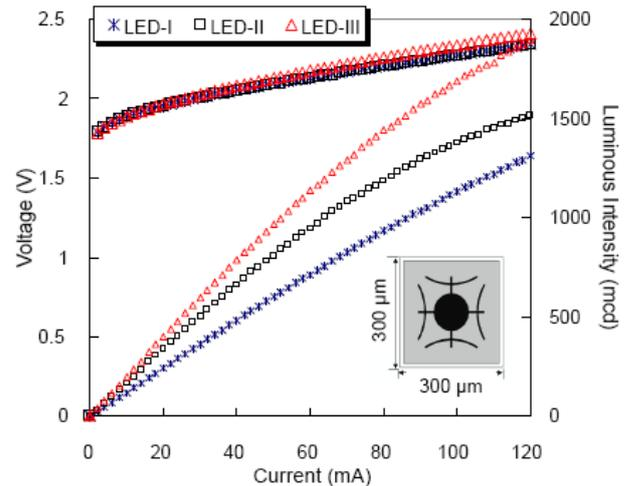
Fig. 4. The corresponding luminous intensity-current-voltage (L-I-V) characteristics of the LED-I, LED-II, and LED-III.
