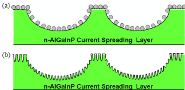
Fig. 2. Schematic diagram of (a) The silica nano-particles were spin-coated on the wafer surface which has bowl-shaped textured. (b) The nano-scale rod was formed on surface after dry-etching process.
