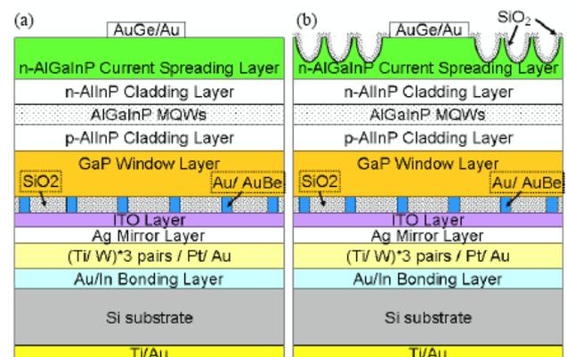
Fig. 1. Schematic diagram of the metal bonding AlGaInP-based LEDs (a) The LED-I device structure has a plane surface. (b) The LED-II device has micro-bowls array texture on surface and the LED-III device is added nano-rods texture in micro-bowls.
