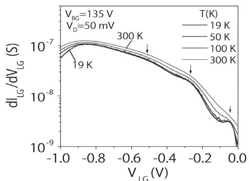
Fig. 5. Temperature dependency of  $dI_{LG}/dV_{LG}$  for devices with SOI thickness of 10 nm at  $V_{BG} = 135$  V and  $V_D = 50$  mV.
