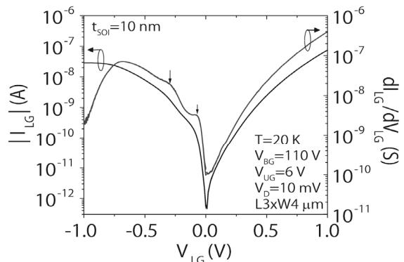
Fig. 3.  $I_{LG}$  and  $dI_{LG}/dV_{LG}$  curve with nominal SOI thickness of 10 nm at 20 K.
