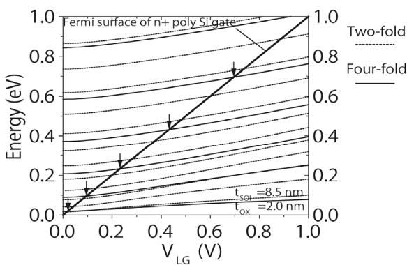
Fig. 6. Calculated energies of subbands as a function of  $V_{LG}$  for  $t_{SOI} = 8.5$  nm and  $t_{ox} = 2.0$  nm. The solid lines and the dotted lines represent the subbands arising from the four-fold and the two-fold valleys, respectively. Arrows indicate coincidence points with the gate Fermi surface and the subbands edge originating from four-fold valleys.
