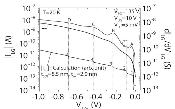
Fig. 7.  $I_{LG}$  and  $dI_{LG}/dV_{LG}$  curve at 20 K for the device with nominal SOI thickness of 10 nm. Calculated  $I_{LG}$  with  $t_{SOI} = 8.5$  and  $t_{ox} = 2.0$  nm are also plotted. Indexes “1” to “5” represent subband-edge of four-fold valleys.
