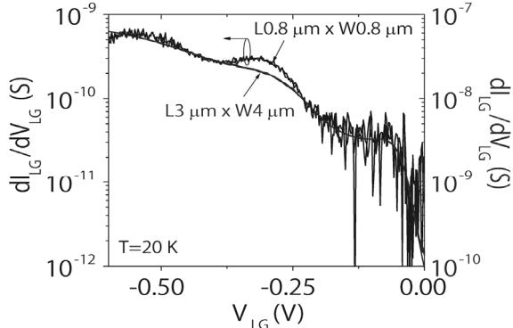
Fig. 4. Tunnel conductance  $dI_{LG}/dV_{LG}$  for ( $L \times W = 3 \times 4 \mu\text{m}$ ) and ( $0.8 \times 0.8 \mu\text{m}$ ) for devices with SOI thickness of 10 nm.
