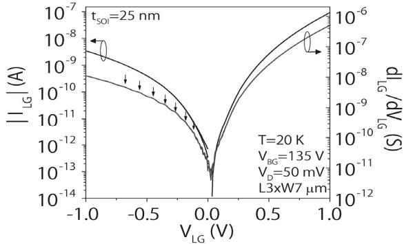
Fig. 2.  $I_{LG}$  and  $dI_{LG}/dV_{LG}$  curve with nominal SOI thickness of 25 nm at 20 K.
