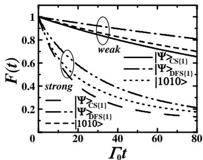
FIG. 2: Time-dependent fidelity of four-qubit states for a cluster state, a DF state, and a product state  $|1010\rangle$ , in case  $\{1\}$ .  $\Gamma_0 = J$ ,  $\Gamma'_i = \Gamma_i$ . The 'weak' indicates a weak measurement case of  $\zeta = 0.2$  and the 'strong' indicates a strong measurement case of  $\zeta = 0.6$ .
