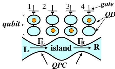
FIG. 1: Four qubits that use double QD charge states are capacitively coupled to a double QPC detector with an island. One excess charge is injected into each qubit. Single energy level is assumed in each QD and the island.
