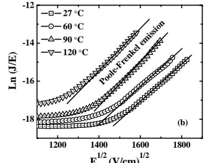
**Fig. 8(a).**  $J-V$  curves of Sm<sub>2</sub>O<sub>3</sub>/SiO<sub>2</sub> capacitors with an 8.5 nm thick Sm<sub>2</sub>O<sub>3</sub> and a 3.5 nm thick SiO<sub>2</sub> measured from 27 to 120 °C. **(b)**  $\ln(J/E)$  versus  $E^{1/2}$  at different temperatures measured at high positive bias. P-F emission likely dominates in this region from the room temperature to 120 °C.
