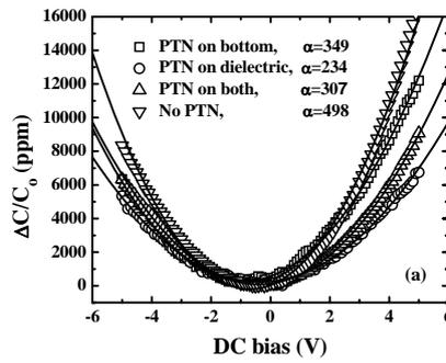
**Fig. 2(a).** Normalized  $C-V$  curves of Sm<sub>2</sub>O<sub>3</sub> MIM capacitors with or without optimized PTN on bottom electrode, dielectrics, and both bottom electrode and dielectrics. **(b)** Summary of the quadratic and linear VCC of Sm<sub>2</sub>O<sub>3</sub> MIM capacitors after different PTN. The best VCCs are obtained by using PTN directly on dielectrics.
