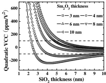
**Fig. 3.** Simulated result of quadratic VCC versus SiO<sub>2</sub> thickness with varying Sm<sub>2</sub>O<sub>3</sub> thicknesses. The quadratic VCC is sensitive to the thicknesses of both SiO<sub>2</sub> and Sm<sub>2</sub>O<sub>3</sub>.
