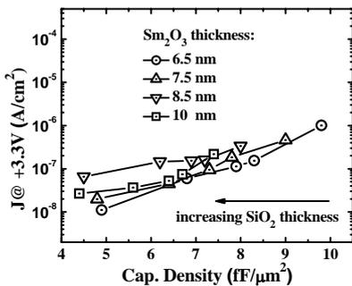
**Fig. 7.** Summary of the leakage current densities of Sm<sub>2</sub>O<sub>3</sub>/SiO<sub>2</sub> MIM capacitors with various combinations of Sm<sub>2</sub>O<sub>3</sub> (6.5, 7.5, 8.5, and 10 nm) and SiO<sub>2</sub> (3 nm to 7 nm) thicknesses.
