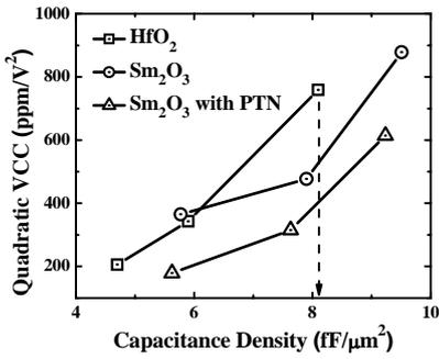
**Fig. 1.** Quadratic VCC ( $\alpha$  value) versus capacitance density of HfO<sub>2</sub> and Sm<sub>2</sub>O<sub>3</sub> (with or without PTN). Sm<sub>2</sub>O<sub>3</sub> MIM with PTN on Sm<sub>2</sub>O<sub>3</sub> dielectrics can obtain much lower quadratic VCC.
