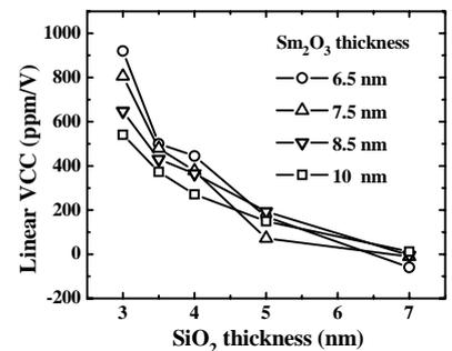
**Fig. 6.** Linear VCC versus SiO<sub>2</sub> thickness with varying the thickness of SiO<sub>2</sub> and Sm<sub>2</sub>O<sub>3</sub>. The linear VCC can be modulated to near zero by increasing the thickness of SiO<sub>2</sub>.
