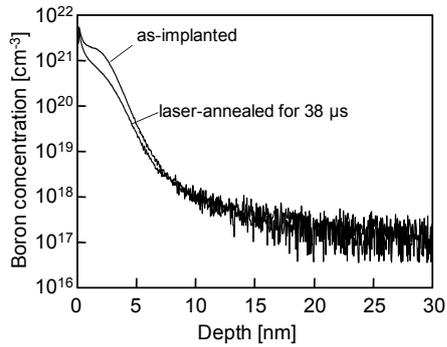
**Fig.3** Boron atoms in-depth profiles for samples as implanted and laser annealed for 40 μs.
