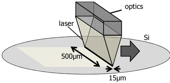
**Fig.1** Schematic image of laser irradiation
