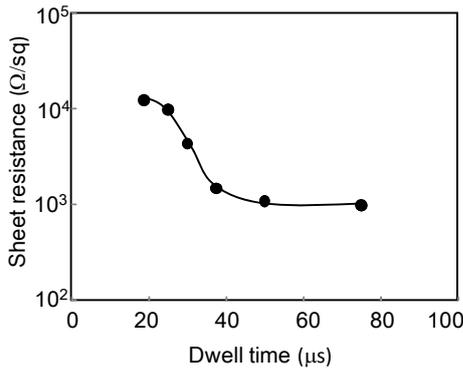
**Fig.2** Sheet resistance as a function of laser dwell time for samples implanted with boron clusters at 6 keV.
