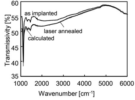
**Fig.4** FTIR transmissivity spectra for samples boron as implanted and laser annealed for 40 μs. A spectrum calculated by a numerical program of free carrier optical absorption was also presented.
