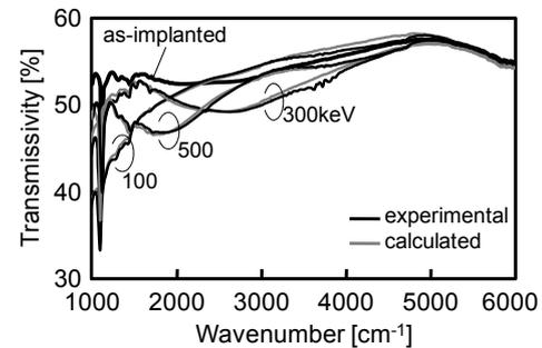
**Fig.6** FTIR transmissivity spectra of the samples as implanted and laser annealed for a dwell time of 43 μs for phosphorus implantation at 100, 300 and 500 keV. Spectra calculated by a numerical program of free carrier optical absorption were also presented.
