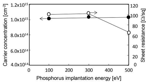
**Fig.7** Carrier concentration and sheet resistance as a function of phosphorus implantation energy for samples implanted with 1x10<sup>15</sup> cm<sup>-2</sup> phosphorus atoms and annealed by laser for 43 μs.
