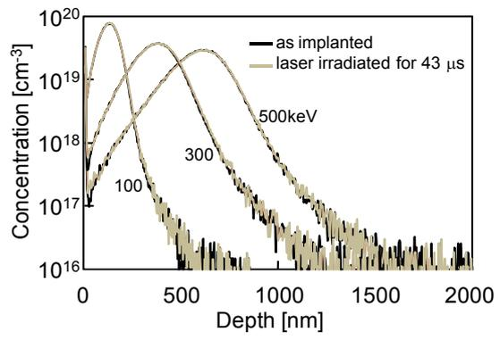
**Fig.5** Phosphorus concentration in-depth profiles for samples as implanted and laser annealed with a dwell time of 43 μs in the cases of implantation at 100, 300 and 500 keV.
