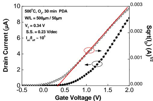
Fig. 7.  $I_D$ - $V_G$  characteristics of ZnO TFTs with the TiHfO gate dielectric annealed at 500°C.
