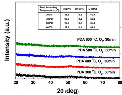
Fig. 4. XRD analysis of TiHfO with different annealing treatment. The inset shows the atomic composition ratio from XPS analysis.
