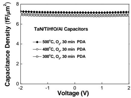
Fig. 2. MIM C-V characteristics of TaN/TiHfO/Al capacitors with the high- $\kappa$  dielectric annealed at different temperatures.
