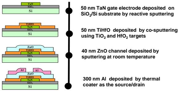
Fig. 1. Schematic cross section diagram and process flow of ZnO TFTs with the high- $\kappa$  TiHfO as dielectric.
