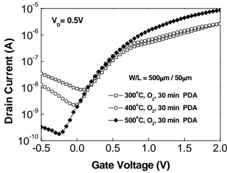
Fig. 5.  $I_D$ - $V_G$  characteristics of ZnO TFTs with the TiHfO gate dielectric annealed at different temperatures.
