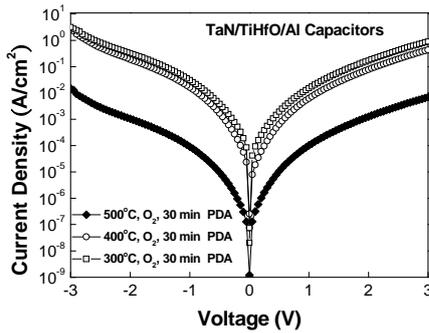
Fig. 3. Leakage current comparison of TaN/TiHfO/Al capacitors for different high- $\kappa$  annealing temperatures.
