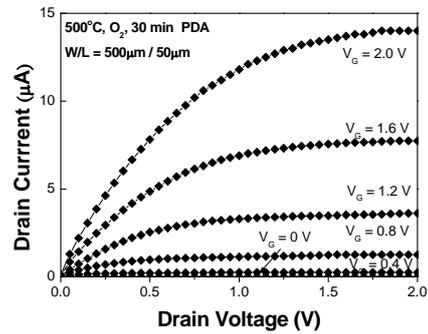
Fig. 6.  $I_D$ - $V_D$  characteristics of ZnO TFTs with the TiHfO gate dielectric annealed at 500°C
