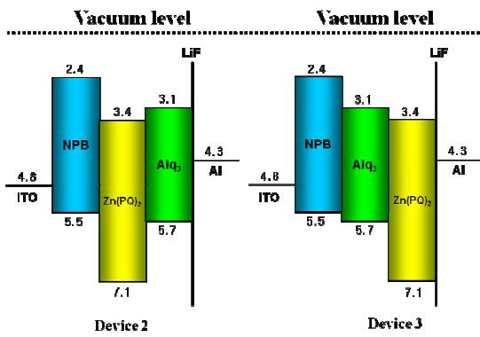
Fig. 2 The energy level alignment of the devices.
