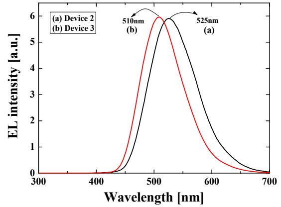
Fig. 4. EL spectrum of the devices 2, 3
