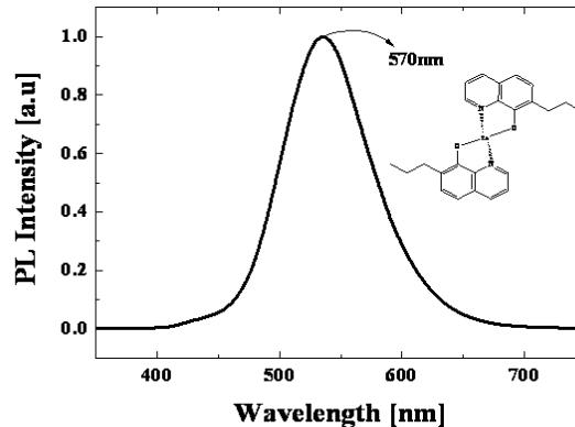
Fig. 1 PL spectrum of Zn(PQ)<sub>2</sub>
