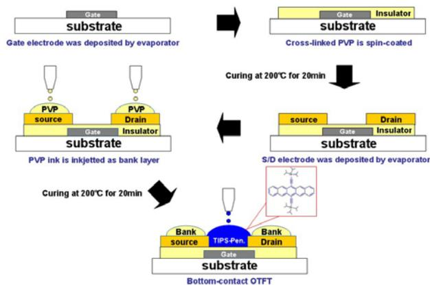
Fig.1. Fabrication process flow and the schematic structures of OTFT
