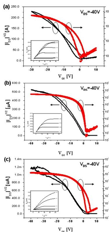
Fig. 3. The electrical characteristics a) without treatment, b) with UV ozone treatment, c) with PVP bank layers for OTFTs fabricated by ink-jet printing method.
