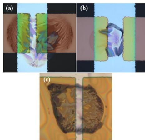
Fig. 2. Crystallized TIPS-pentacene on channel a) without treatment, b) with UV ozone treatment, c) inkjet printed TIPS-pentacene inside PVP bank layer
