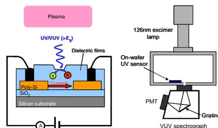
Figure 1 (a) Schematic illustration of the on-wafer UV sensor (b) Schematic illustration of the UV/VUV spectrum observation.
