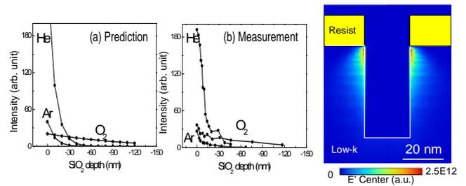
Figure 4. Depth profile of E' Center defect densities (a) predicted results, (b) measured results by ESR.
