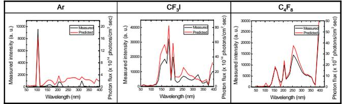
Figure 3. Predicted profiles of UV/VUV spectrum for Ar, CF<sub>3</sub>I, and C<sub>4</sub>F<sub>8</sub> plasmas.
