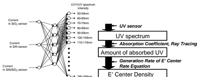
Figure 2. (a) Neural network system for the prediction of UV/VUV spectrum (b) Sequence of calculation of E' Center density.
