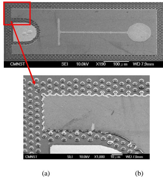
Fig. 1 SEM images of (a) full view and (b) enlarge view of the LED IV with textured side wall and  $\mu$ -pillars..
