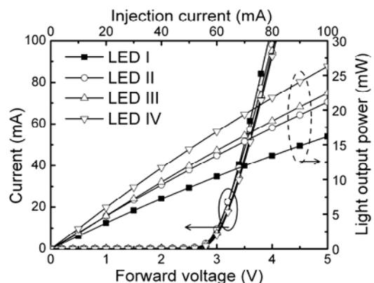
Fig. 2 L-I-V characteristics of the fabricated LEDs.
