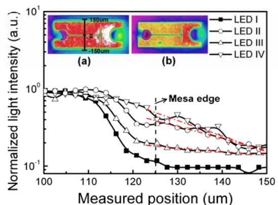
Fig. 3 The light intensity profiles crossed the LEDs at 20mA of all LED samples. Insets show the light intensity image of (a) LED II and (b) LED I.
