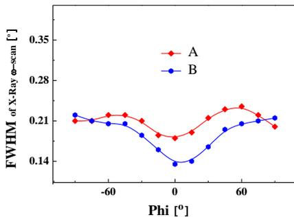
Fig 2. FWHM of HR-XRD (11-20)  $\omega$ -scans for sample A and sample B which respect to the in-plane beam orientation
