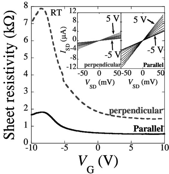
Fig.2 Sheet resistivity as a function of gate voltage observed in the transistor with 2- $\mu\text{m}$ -length and 0.3- $\mu\text{m}$ -width of the channel. The inset shows  $I_{SD}$  vs  $V_{SD}$ . The applied gate voltage is from -5 V to 5 V at 1 V step. The solid line is obtained in the parallel-channel FET and the dashed is in the perpendicular-channel FET.
