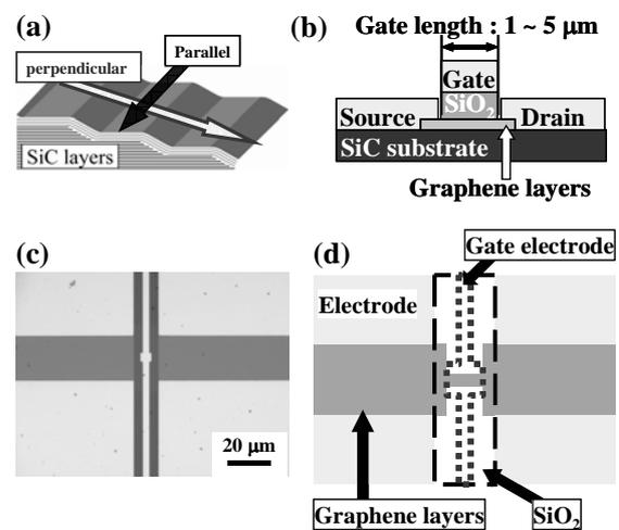
Fig. 1 (a)Schematic of vicinal SiC surface with current flow directions in step structures. (b)Cross-sectional schematic image of graphene FET. (c)Optical microscope image of the FET in four-terminal configuration. (d)Schematic image of the FET.
