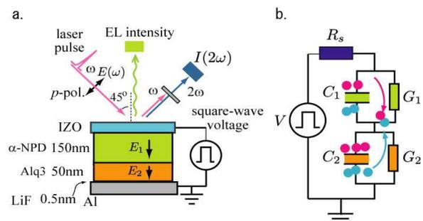
Fig. 1 (a) OLED (IZO/ $\alpha$ -NPD/Alq3/LiF/Al) structure and experimental arrangement for EFISHG measurements. (b) Equivalent circuit model for OLED based on the Maxwell-Wagner effect.
