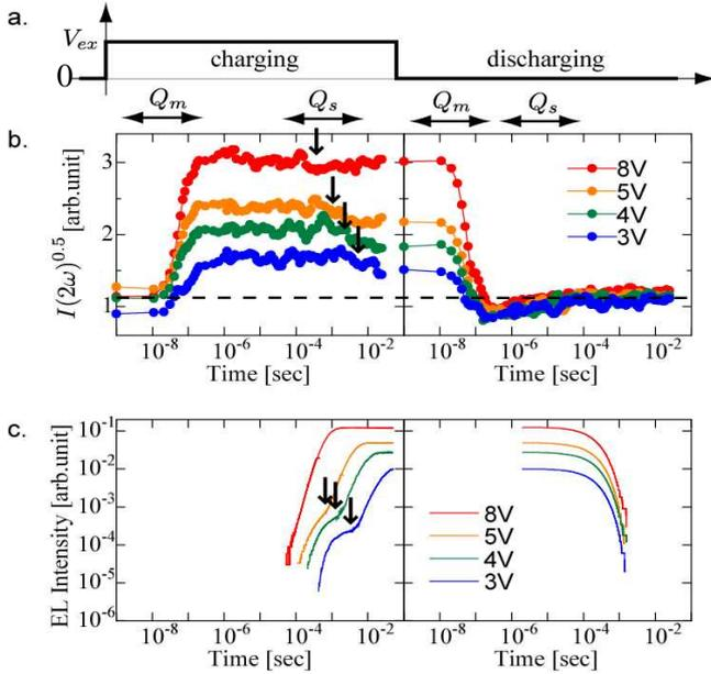
Fig.2 (a) Square-wave voltage applied for OLED. (b) EFISHG transient  $I(2\omega)^{0.5}$  proportional to electric field in  $\alpha$ -NPD layer  $E_1$  only. (c) Transient EL measurements.
