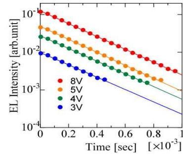
Fig.3 Semi-log plots of EL decay after shot-circuited. Voltage applied for charging was indicated.
