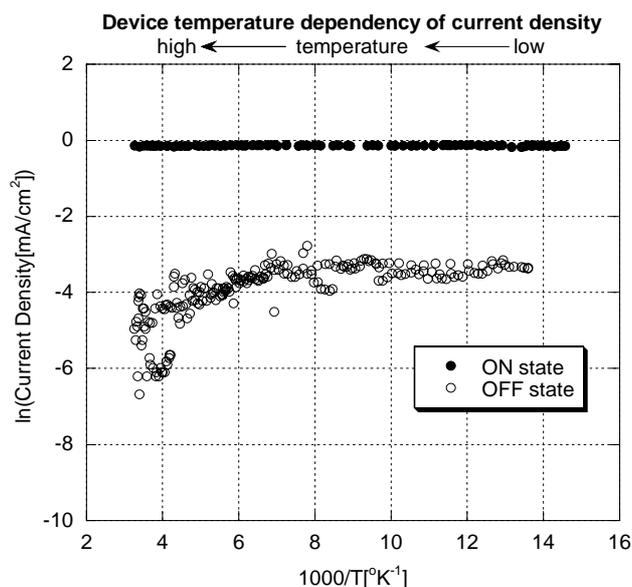
Fig. 3 The Arrhenius plot of changes of the current density accompanying the device temperature. ON state (filled circle) is independent of the device temperature.
