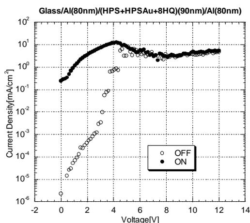
Fig. 2 Typical J-V characteristics of the OBD using HPS and HPSAu. This device shows two stable states (ON and OFF) of electrical conductivity in the voltage regions from 0V to 4V.
