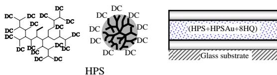
Fig. 1 Schematic structure of HPS and the OBD. DC indicate dithiocarbamate endgroup.
