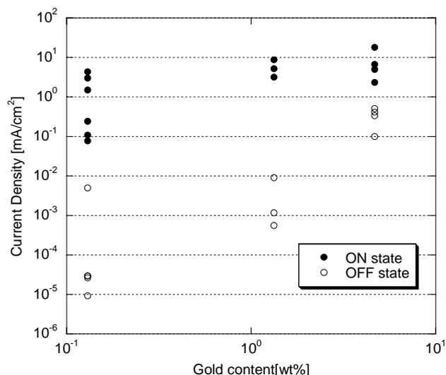
Fig. 4 The dependency of the current density on the gold content in organic composite films. Some devices were fabricated with the respective content and the ON current density and the OFF current density of them were plotted. One circle (filled and empty) exhibits ON state and the OFF state of one device.
