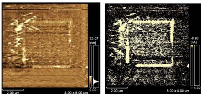
Figure 5. AFM height image and current-map image after the application of bias voltages
