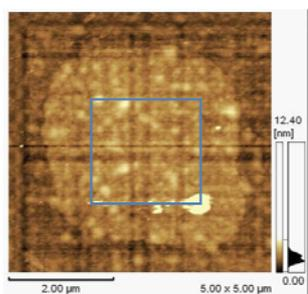
Figure 3. AFM height image of cross-linked/doped precursor polycarbazole film after the application of 5 V
