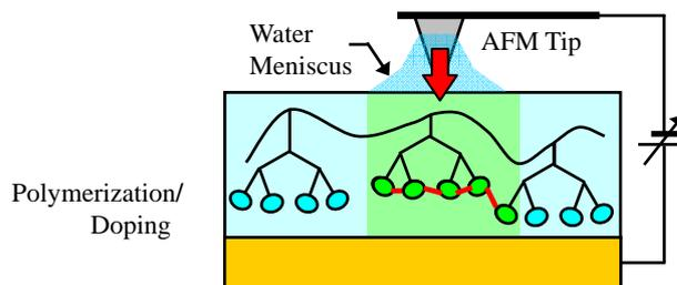
Figure 2. AFM nanolithography used in this study
