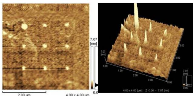
Figure 4. AFM height image after dots are processed by AFM nanolithography
