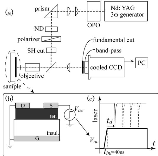
Fig. 1: experimental setup for SHG measurement
