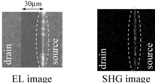
Fig. 4: spatial distribution of EL and SH intensity responsible for this EL enhancement. Results evidently showed that there are two kinds of EL from the tetracene. The EL enhanced around 620nm was our main interest here.
