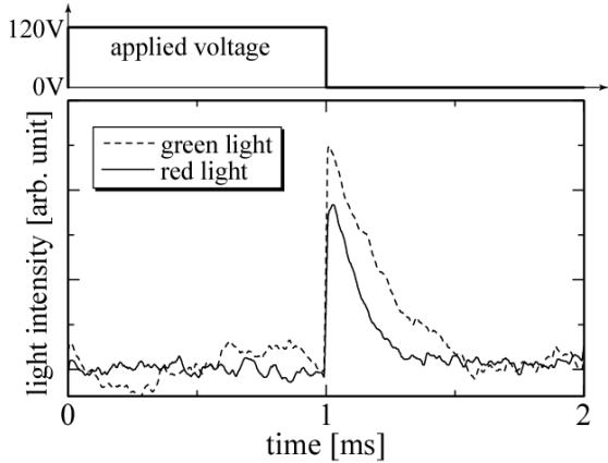
Fig. 3: time dependence of EL intensity
