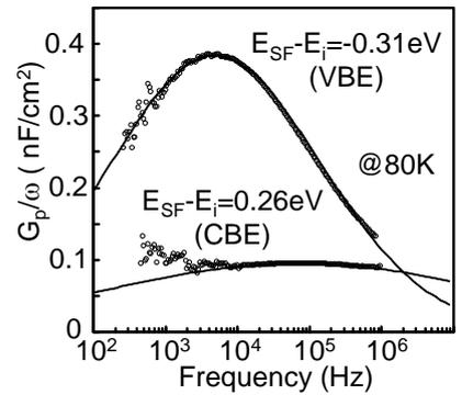
Fig. 9: Conductance curves measured at near CBE and VBE.
