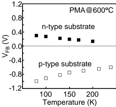
Fig. 7: Dependence of  $V_{FB}$  on measurement temperature for the capacitor with PMA at 600°C.
