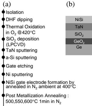
Fig. 1 (a) Fabrication process flow of the capacitors and (b) the gate stack structures of the fabricated capacitors.
