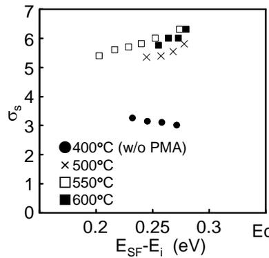
Fig. 5: Energy distributions of  $\sigma_s$  for the capacitors with various PMA temperatures. Here,  $\sigma_s$  is represented in the unit of  $kt/q$ , where  $k$ ,  $T$  and  $q$  are the Boltzmann's constant, the absolute temperature, the elementary charge, respectively.
