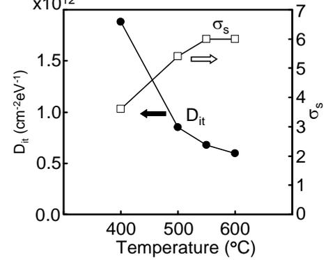
Fig. 6: PMA temperature dependence of  $D_{it}$  and  $\sigma_s$ .  $D_{it}$  and  $\sigma_s$  were evaluated at  $E_{SF}-E_i=0.26eV$ .
