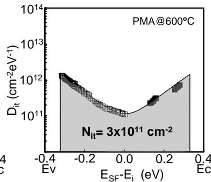
Fig. 11: Energy distributions of  $D_{it}$  for the capacitor with PMA at 600°C evaluated from the conductance method.
