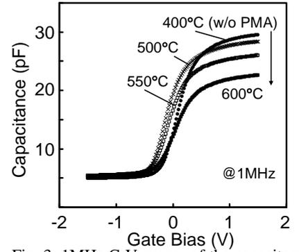
Fig. 3: 1MHz C-V curves of the capacitors with various PMA temperatures measured at room temperature.
