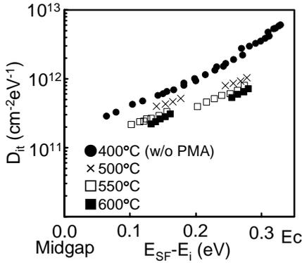
Fig. 4: Energy distributions of  $D_{it}$  for the capacitors with various PMA temperatures. Here,  $E_{SF}$  and  $E_i$  are Fermi level at a Ge surface, intrinsic Fermi level of Ge, respectively.
