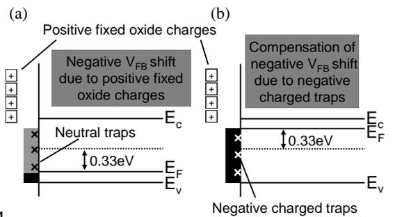
Fig. 12: Schematic diagram of the relationship between the location of interface charges and the nature of interface traps for (a) p-type and (b) n-type substrates at 80K.
