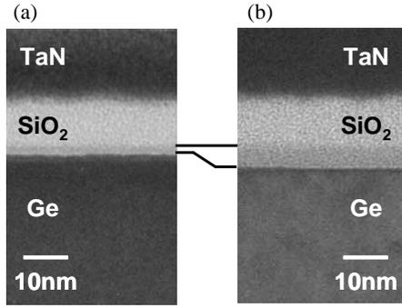
Fig. 2: TEM images of the fabricated capacitors (a) without and (b) with PMA at 600°C.
