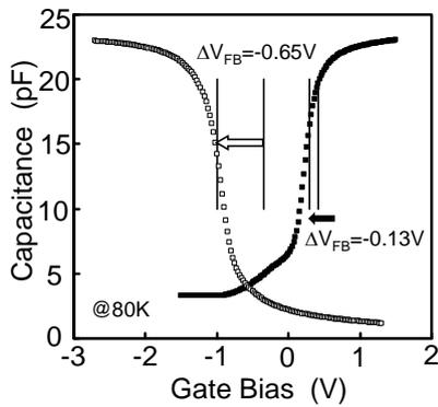
Fig. 8: 1MHz C-V curves of the capacitors with p- and n-type substrates measure at 80K.
