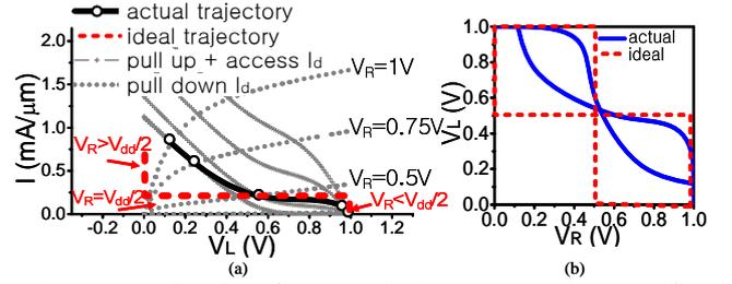
Figure 3 (a) **Read trajectory**. Circles correspond to specific points at  $V_R=0, 0.25, 0.5, 0.75, 1V$  biasing conditions. Ideal trajectory has three segments: infinite slope and small  $V_L$  at  $V_R > V_{dd}/2$  biasing; zero slope at  $V_R = V_{dd}/2$  biasing; infinite slope and large  $V_L$  at  $V_R < V_{dd}/2$  biasing. (b) **Read butterfly curve**.
