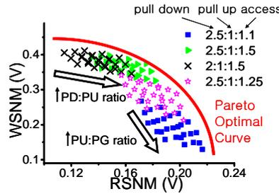
Figure 7 **RSNM vs. WSNM** with different ratios of the widths of transistors (cell area less than 10 times of the pull up transistor's area). Pareto optimal curve are composed of the points that there is no design with both WSNM and RSNM larger than these points.
