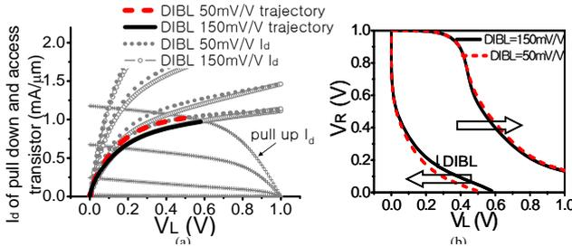
Figure 5 (a) **Write trajectory** for different DIBLs of the access transistor. Low DIBL reduces the  $V_L$  of trajectory points at the same  $V_R$  biasing and leads to larger WSNM. (b) **Write voltage transfer curve** for different DIBLs of access transistor.
