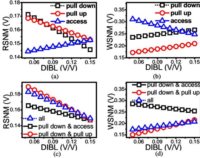
Figure 2 **DIBL vs. SNM**. (a), (b) adjust DIBL of a single transistor. (c), (d) adjust DIBL of multiple transistors for the half cell. In (a), changing pull down is most effective in improving RSNM (17.6%); and in (b) changing access is most effective for WSNM (25.1%).
