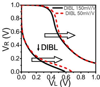
Figure 6 **Write voltage transfer curves** for different DIBLs of pull up transistor.
