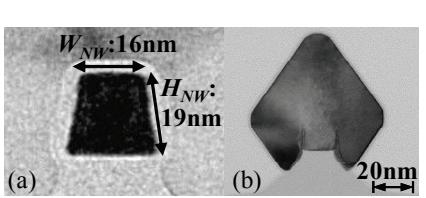
Fig.3 Typical cross-sectional TEM images: (a) nanowire and (b) S/D after epi-Si NW with NW height ( $H_{NW}$ ) and width ( $W_{NW}$ ) of 19nm and 16nm was successfully fabricated.
