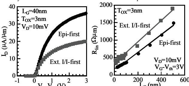
Fig.4  $I_D - V_G$  of Epi-first and Ext. I/I-first NW FETs.  $I_D$  is normalized by circumference ( $W_{NW} + 2 \cdot H_{NW}$ ).
