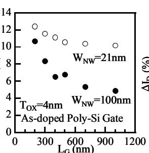
Fig.12  $L_G$  dependence of  $I_D$  enhancement of high-to-low-dose gate NW FETs.
