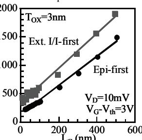
Fig.5 Typical  $R_{lin}$ - $L_G$  plots, where  $L_G$  is defined as gate ploy-Si length.
