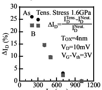
Fig.17  $L_G$  dependence of  $\Delta I_D$  induced by tensile strain.
