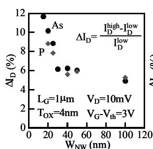
Fig.11  $W_{NW}$  dependence of  $I_D$  enhancement of high-to-low-dose gate NW FETs.
