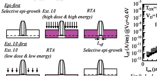
Fig.6 Schematics of Epi-first and Ext. I/I-first processes.
