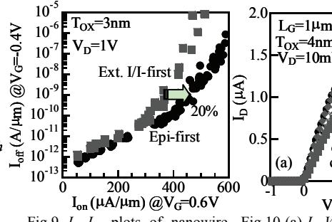
Fig.9  $I_{on}$ - $I_{off}$  plots of nanowire FETs. 20%  $I_{on}$  enhancement is achieved at  $I_{off}$  of 1nA/μm.
