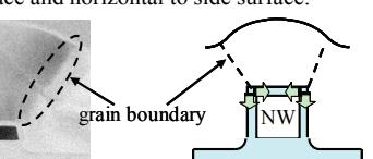
Fig.15 Cross-sectional TEM image of NW FETs. Poly-Si grain boundary at the corner could induce outward stress.
