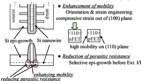
Fig.1 Schematics of top and cross-sectional view of nanowire FETs. S/D and heavily-doped Poly-Si gate. Mobility enhancement and resistance reduction are required.
