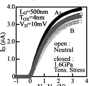
Fig.16  $I_D - V_G$  characteristics with or without tensile SiN liner.  $H_{NW} = 14\text{ nm}$ .  $W_{NW} = 21\text{ nm}$ .
