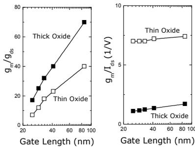
**Fig. 10** Excellent analog operation is possible down to  $L_G=25$  nm and without need to special design [1].
