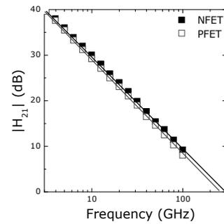
**Fig. 9** ETSOI NFETs and PFETs with  $L_G=25$  nm and  $CPP = 260$  nm show  $f_T$  of 300 and 260 GHz, respectively.
