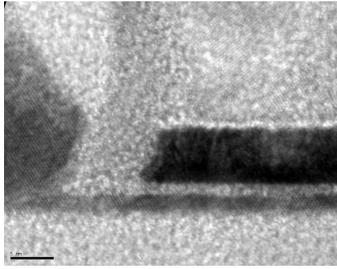
**Fig. 1** TEM cross section of the ETSOI device with a channel thickness of 1.9 nm.
