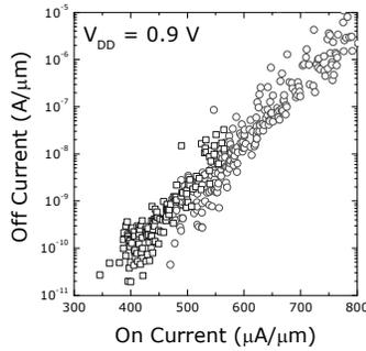
**Fig. 8**  $I_{on}$ - $I_{off}$  characteristics of LP and HP PFETs showing drive current of 480 and 660  $\mu A/\mu m$  at  $I_{off} = 1$  and 100 nA/ $\mu m$ , respectively.
