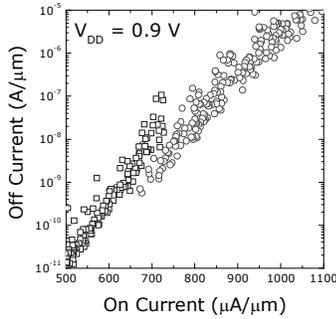
**Fig. 7**  $I_{on}$ - $I_{off}$  characteristics of LP and HP NFETs showing drive current of 650 and 870  $\mu A/\mu m$  at  $I_{off} = 1$  and 100 nA/ $\mu m$  off current, respectively.
