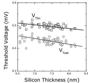
**Fig. 12** Correlation between channel thickness and short channel  $V_T$  showing 25 mV/nm sensitivity.
