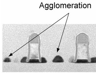
**Fig. 2** TEM cross section showing agglomeration with non-optimized epitaxy process.
