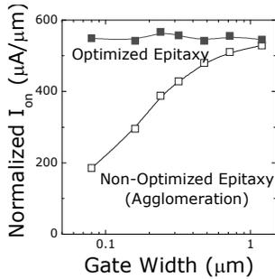
**Fig. 4** Drive current at constant overdrive showing the importance of epitaxy optimization to avoid agglomeration in narrow devices.
