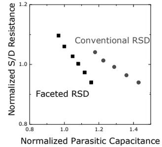
**Fig. 6** TCAD simulations showing 15% reduction  $C_{para}$  by faceted RSD at a constant  $R_{ext}$  [1].
