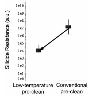
**Fig. 3** Significant reduction in silicide resistance indicates that low-temperature pre-clean is needed to avoid agglomeration.
