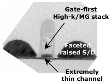
**Fig. 5** TEM cross section of the ETSOI device.
