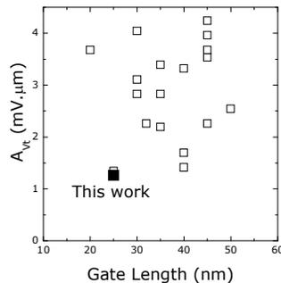
**Fig. 11** Record device matching is achieved in ETSOI devices with undoped channel [1].
