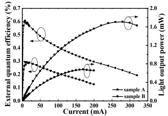
Fig. 5.  $L$ - $\eta_{EQE}$ - $I$  characteristics of sample A and B as a function of injection current
