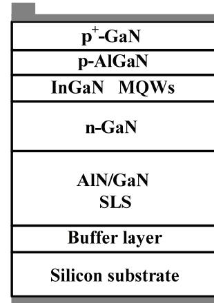
Fig. 1. Schematic structure of GaN-based LEDs
