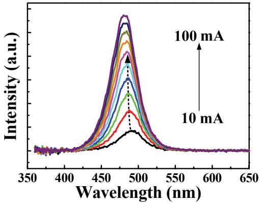
Fig. 4. EL spectra of sample A as a function of injection current!
