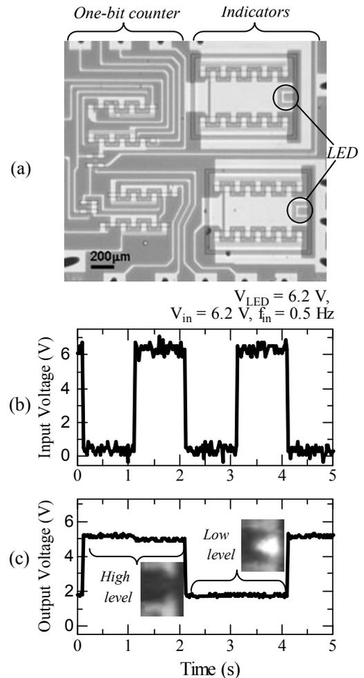
Fig. 3 Optical micrograph and device performance of one-bit counter circuits with LEDs. (a) micrograph of fabricated chip, (b) input voltage timing chart, and (c) output voltage timing chart with the snapshot of LED taken at 0.5 Hz.
