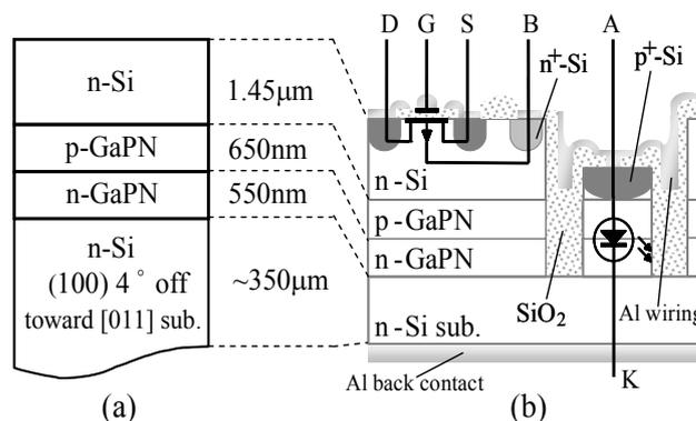
Fig. 1 Schematic images of (a) Si/GaPN/Si layer structure, and (b) cross section of p-MOSFET and LED fabricated in a Si/GaPN/Si heterostructure.
