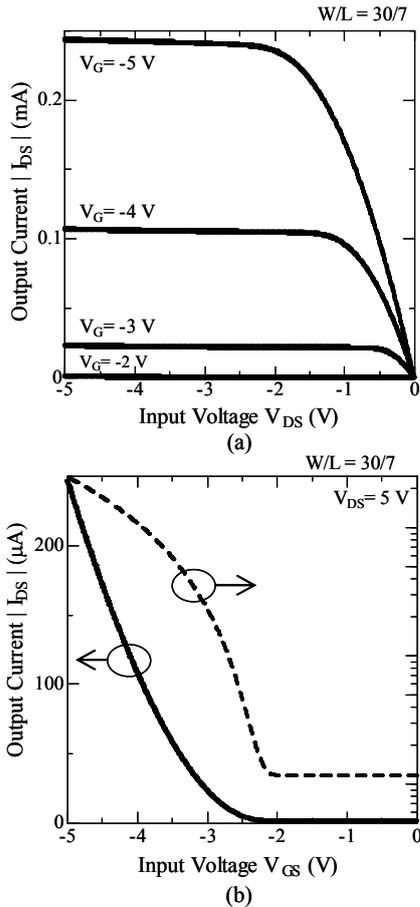
Fig. 2 Typical device characteristics of p-MOSFET. (a)  $I_{DS}$ - $V_{DS}$  characteristics with the  $V_G$  changing from -5 to 0 V and (b)  $I_{DS}$ - $V_{GS}$  characteristics with the  $V_{DS} = 5$  V.
