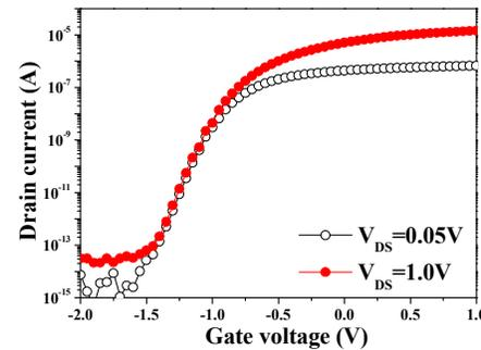
Fig. 8 Measured  $I_D(V_G)$  of 15-nanowire JL MuGFETs with  $W_{mask}=50nm$  and  $L_{gate}=1\mu m$ .
