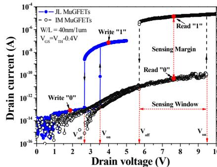
Fig. 5: Measured drain current hysteresis characteristics of JL and IM MuGFETs with  $V_{GS}=V_{TH}+0.4V$  (single nanowire).
