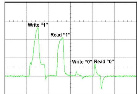
Figure 12 – Measured source current during cell operation for JL MuGFETs device with  $W_{mask}=50nm$  and  $L_{gate}=1\mu m$ .
