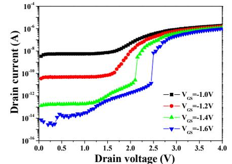
Fig. 9 Measured  $I_D$ - $V_D$  characteristics of the JL MuGFETs device at different gate voltages.
