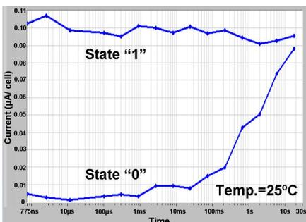
Fig. 10: Measured retention characteristics of the JL MuGFETs device at room temperature.
