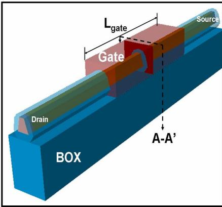
Fig. 1: 3-dimensional schematic view of the junctionless MuGFETs device.
