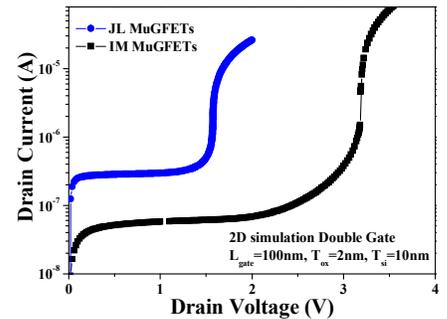
Fig. 6: Simulated  $I_D$ - $V_D$  characteristics of JL and IM double-gate device with  $L_{gate}=100nm$ ,  $T_{si}=10nm$ ,  $T_{ox}=2nm$ .
