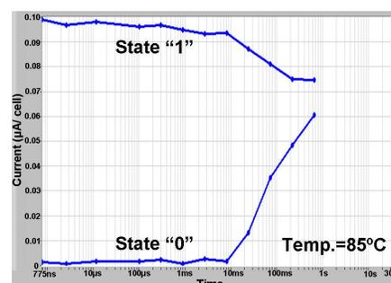
Fig. 11: Measured retention characteristics of the JL MuGFETs device at 85°C.
