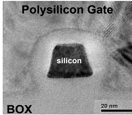
Fig. 2: cross-sectional high-resolution TEM photograph along A-A' direction in fig.1.
