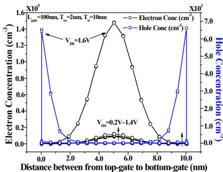
Fig. 7 Simulated electron concentration and hole concentration in JL double-gate device at center of channel from top-gate to bottom-gate for different drain voltage values.
