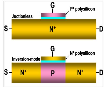
Fig. 3 Schematic view of junctionless and inversion-mode n-channel devices.
