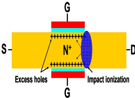
Fig. 4: cross-sectional schematics of possible causes of latch-up in JL double-gate devices.
