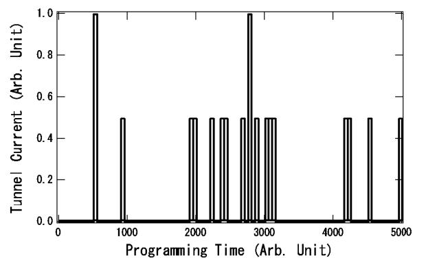
**Fig. 6** The dependency of tunneling current on the programming time with proposed collective tunneling model.
