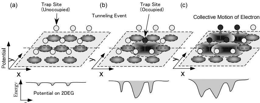
**Fig. 3** The potential profiles in the suggested tunneling model. a) Unoccupied state, b) first electron tunneling, c) collective tunneling.
