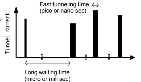
**Fig. 4** The dependency of tunneling current on the programming time induced by proposed rare events.
