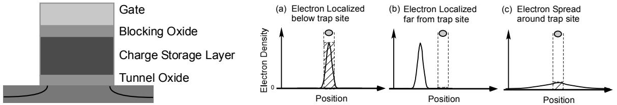
**Fig.1** Schematic illustration of SONOS type NVM cell structure
