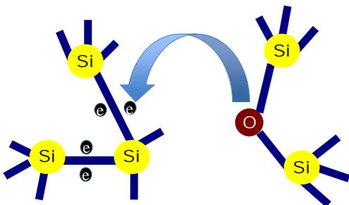
Fig. 10: Schematic view of stabilization mechanism of a N vacancy with an O atom without H incorporation. One electron is supplied from O to form a new Si-Si bond.
