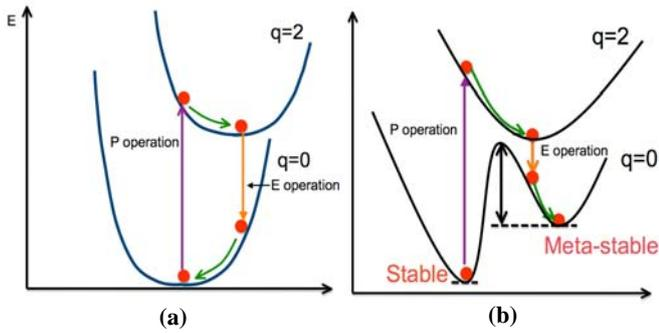
Fig. 1: Schematic illustration of two types of structural changes. (a) Reversible structural change during P/E cycles. (b) Irreversible structural change during P/E cycles. By program and erase operations, the most stable original structure changes into different meta-stable one [Ref 1].
