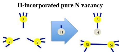
Fig. 6: H-incorporated pure N vacancy model. One dangling bond is terminated by a H atom, and other two dangling bond form a new Si-Si bond.
