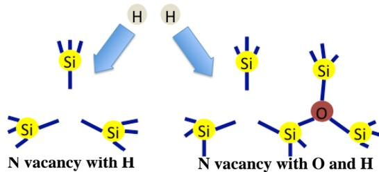
Fig. 4: Atomistic structures of our studied defect models. (Left) A pure N vacancy. (Right) A N vacancy with one substitutional O atom at a N site. We investigated H atom incorporation effect in each N vacancy model.
