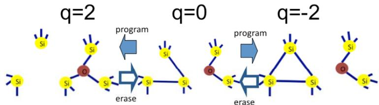
Fig. 11: The atomistic structural change of a N vacancy with one substitutional O atom during P/E cycles (Injection and removal of electron and holes). Structural change is reversible. This N vacancy also has high P/E cycle endurance
