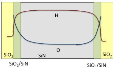
Fig. 3: H and O profiles in MONOS structures. A lot of H atoms are observed in SiN layer [Ref.2] and many O atoms are located at SiN/SiO<sub>2</sub> interfaces [Ref.3].
