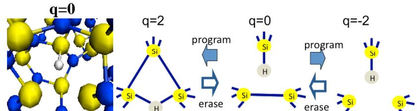
Fig. 7: (Left) Atomistic structures of a H-incorporated pure N vacancy. (Right) Atomistic structure change during P/E cycles (Injection and removal of electron and holes). Structural change is reversible, and high P/E cycle endurance of a N vacancy is maintained.
