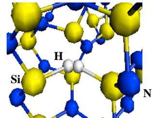
Fig. 5: N vacancy structure with two H incorporation. In this case, H-H distance is shorter than 0.5 Å.
