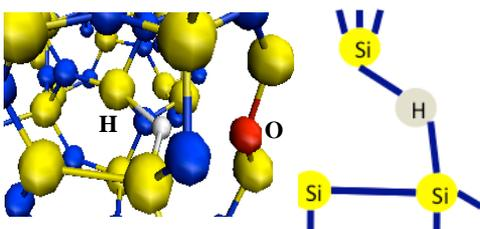
Fig. 8: Atomistic structures of a H-incorporated N vacancy with O atom. Schematic illustration is also shown
