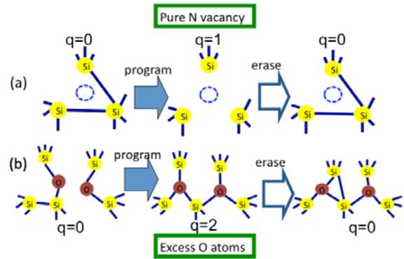
Fig. 2: Examples of reversible and irreversible structural changes during P/E cycles (a) Pure N vacancy reveals reversible change. (b) Defects with two substitutional O atoms at N sites structure has irreversible structural change (Not good for memory properties).
