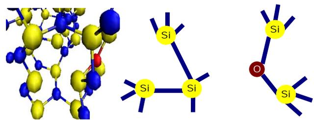
Fig. 9: Atomistic structure of a N vacancy with an O atom without H incorporation. Schematic illustration is also shown.
