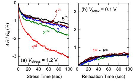
Fig. 3 Change of the resistance shifted during each (a) stress and (b) relaxation stage. The data shown in Fig. 2 are replotted here. The resistance shift  $\Delta R$  are normalized to the sample initial resistance  $R_0$ .
