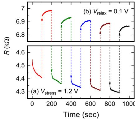
Fig. 2 Resistance drift as a function of time measured with applying (a)  $V_{\text{stress}} = 1.2$  V and (b)  $V_{\text{relax}} = 0.1$  V. On/off cycles were repeated for 5 times.
