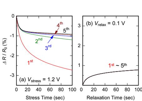
Fig. 6 Simulated resistance drift to reproduce the experimental data shown in Fig. 3. The fitting parameters assumed were, for the stress stage:  $\tau_1 = 2$  s,  $\tau_N = 2 \times 10^5$  s,  $\beta F/k = 0.07$ , and for the relaxation stage:  $\tau_1 = 2$  s,  $\tau_N = 2 \times 10^{16}$  s,  $\beta F/k = 0.07 \times (J_{\text{relax}}/J_{\text{stress}})$ .
