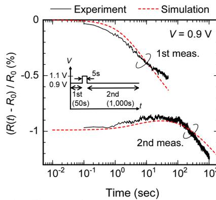
Fig. 7 Experimental and simulated resistance drift. Firstly, the resistance drift was monitored for 50 s under  $V = 0.9$  V, and then the higher voltage of 1.1 V was applied for 5 s. After that, the resistance drift at  $V = 0.9$  V was measured again.
