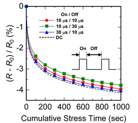
Fig. 8 Simulated results for the on/off ratio dependence of resistance drift under unipolar pulsed stress conditions. The parameter set used is the same as for Fig. 6.
