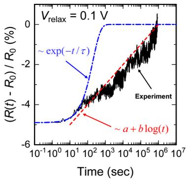
Fig. 4 Long time behavior of the resistance relaxation after applying  $V_{\text{stress}} = 1.2$  V. The data cannot be fitted by the exponential decay curve with a single time constant, but can be well characterized by a logarithmic relation:  $a + b \log(t)$  [1].
