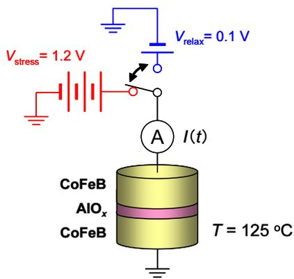
Fig. 1 Schematic view of the experimental method used in this study.
