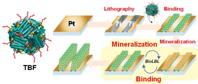
Fig.2. Process flow of Bio-LBL method.
