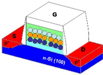
Fig.1. Structure of floating gate memory with multi-layered BND array
