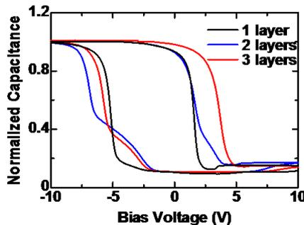
Fig.7. C-V characteristics of the MOS capacitors with multi-layered Ni-BND array
