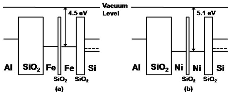
Fig.10. Band diagrams of the MOS capacitors with double-layered (a) Fe-BND array and (b) Ni-BND array
