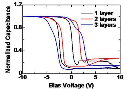
Fig.5. C-V characteristics of the MOS capacitors with multi-layered Fe-BND array
