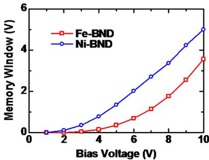
Fig.9. Memory windows of the MOS capacitors with double-layered Fe-BND and Ni-BND array
