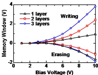
Fig.6. Memory windows of the MOS capacitors with multi-layered Fe-BND array
