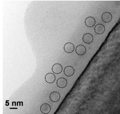
Fig.4. A cross section TEM image of the MOS capacitor with multi-layered
