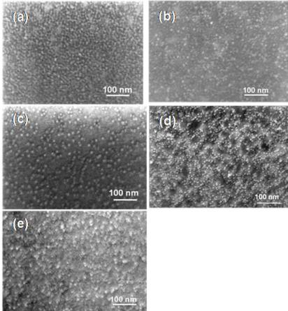
Fig.3. SEM images of (a) TBF adsorbed on tunnel oxide. (b) TBF adsorbed on first SiO<sub>2</sub> interlayer. (c) First SiO<sub>2</sub> interface layer. (d) TBF adsorbed on second SiO<sub>2</sub> interface layer. (e) Second SiO<sub>2</sub> interface layer
