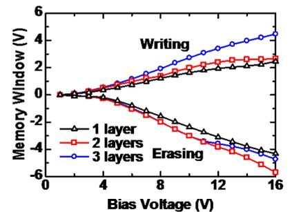
Fig.8. Memory windows of the MOS capacitors with multi-layered Ni-BND array
