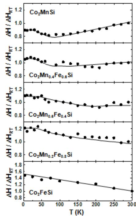
Fig. 2 Temperature dependence of  $\Delta H$  for  $\text{Co}_2\text{Fe}_x\text{Mn}_{1-x}\text{Si}$  films.
