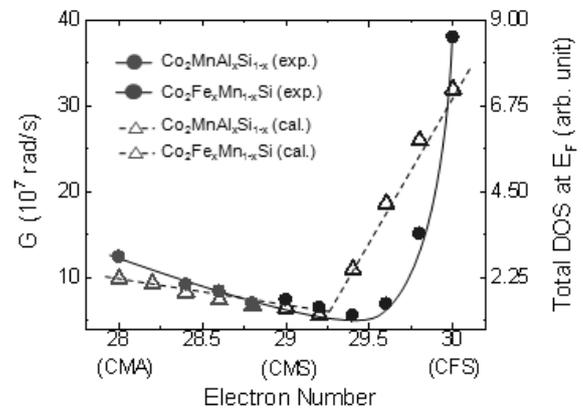
Figure 1 Valence electron number dependence of the Gilbert damping constant (solid line) and calculated density of states at Fermi energy (dashed line) for  $\text{Co}_2\text{MnAl}_x\text{Si}_{1-x}$  and  $\text{Co}_2\text{Fe}_x\text{Mn}_{1-x}\text{Si}$  Heusler alloy films.
