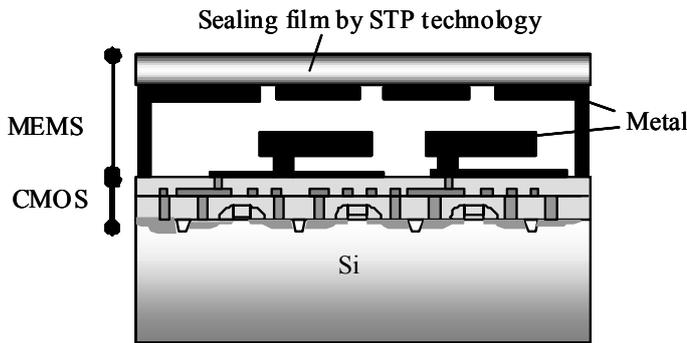
Fig.2. The integrated CMOS-MEMS device structure.
