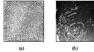
Fig. 6 Fingerprint images of a finger wetted with water captured by (a) the MEMS and (b) a capacitive fingerprint sensor.
