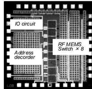
Fig. 8. Fabricated SP8T switch.
