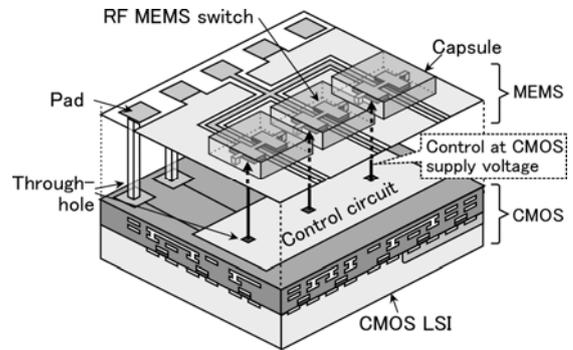
Fig. 7. Schematic of the RF CMOS-MEMS switch. RF MEMS switches are stacked on a CMOS LSI and controlled by a control circuit at the CMOS supply voltage.
