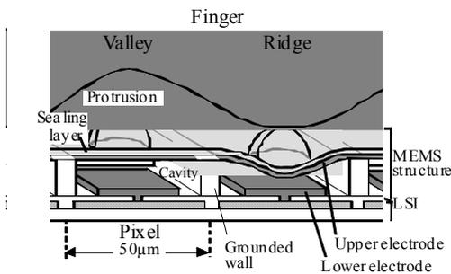
Fig.4. Structure and sensing mechanism of proposed MEMS fingerprint sensor.
