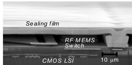
Fig.9 SEM photograph of the SP8T switch.
