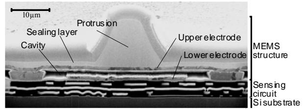
Fig. 5. FIB (Focused Ion Beam) cross section of the pixel.
