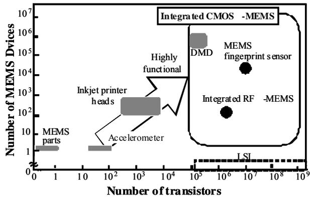
Fig.1. Business trend and correlation between the number of MEMS devices and transistors.
